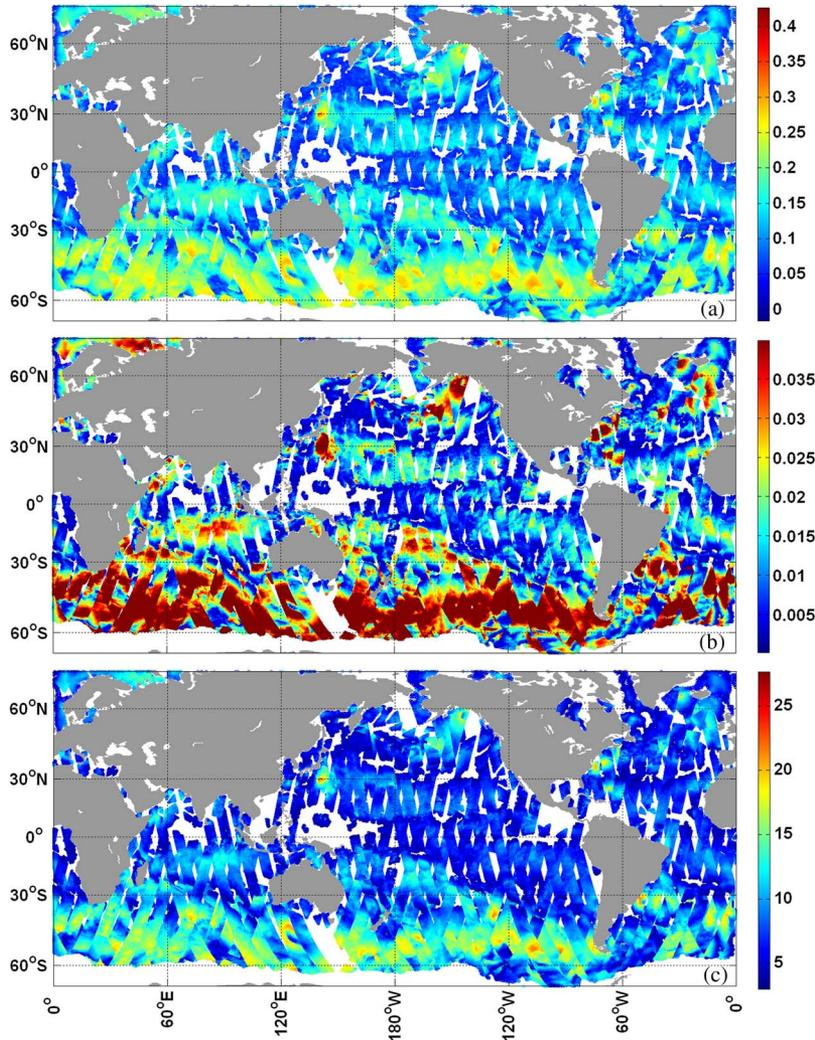
Fig. 2. (a) Distributions of wave steepness ( $\delta$ ) derived from ERS-2 data, (b) distribution of equivalent Charnock parameter  $f(\delta)^2$  using (6), and (c) distributions of wind speed (in meters per second) over the global oceans from August 27 to 29, 1998.
