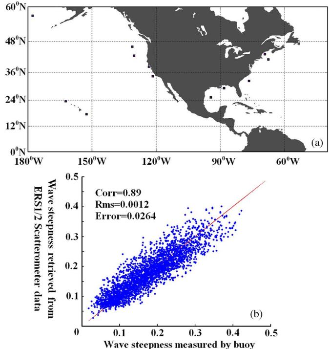
Fig. 1. (a) Distributions of buoys in the (diamonds) North Pacific and North Atlantic Ocean and (b) comparison of  $\delta$  between the buoy records and those retrieved from ERS-1/2 data.
