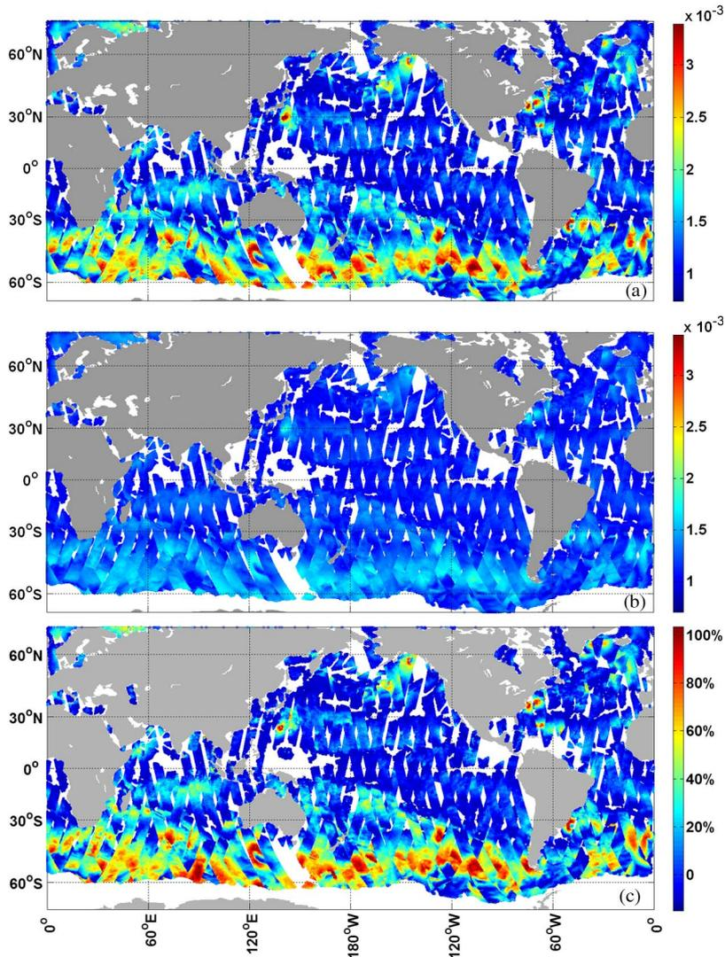
Fig. 3. (a) Distribution of  $C_{DN}$  based on wind speed and wave steepness, (b) distribution of  $C_{DC}$  calculated from wind speed and a constant  $\alpha = 0.011$  proposed by Smith *et al.* [24], and (c) distribution of the percentage  $(C_{DN} - C_{DC})/C_{DC} \times 100\%$ .
