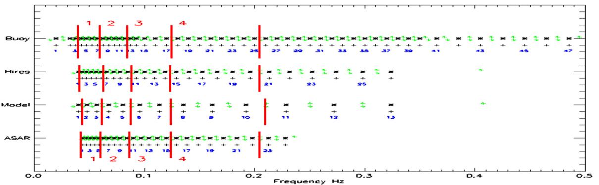
Fig.1. Definition of the 4 frequency bins for comparison of model and observed ocean wave energy spectra.
