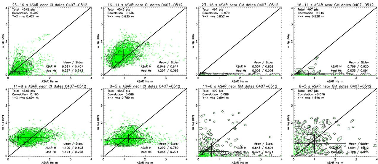
Fig.5. Comparison of model and Envisat ASAR 4-bin wave energy near the CI and GM buoy sites.
