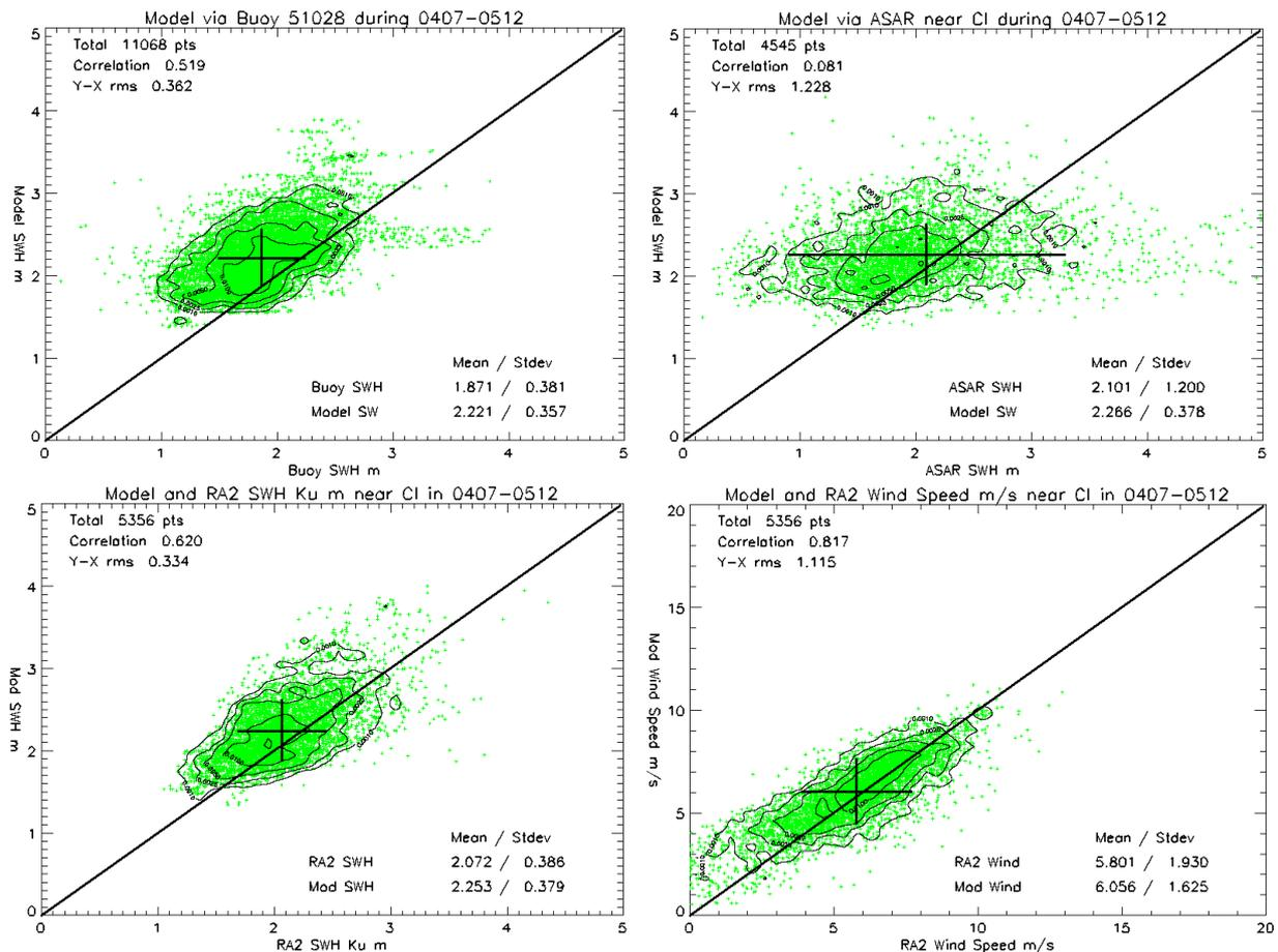
**Fig.2. Comparison of model results with the CI buoy and Envisat measurements near the CI buoy site.**
