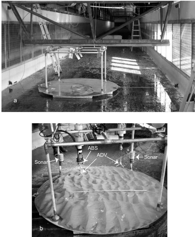
**Figure 1.** (a) Flume and oscillating plate and (b) oscillating plate with instruments, at the end of run 16.
