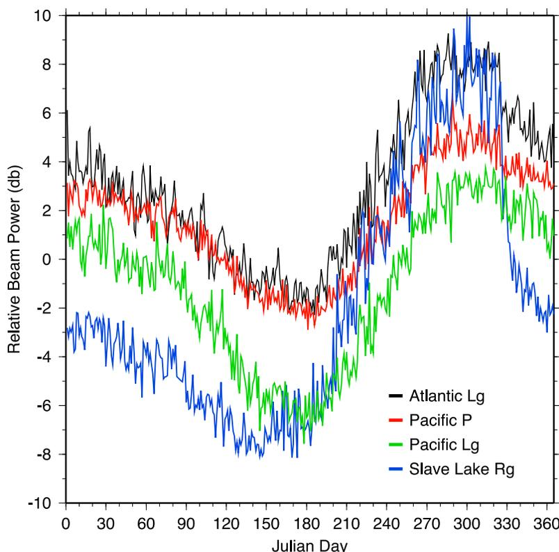
**Figure 10.** Annual variation in four of the noise sources observed at YKA. Each point on a curve is the median noise value for a given julian day from a beam steered toward a specific noise source. In all four cases the beams were bandpassed at 0.3–0.6 Hz with a 4-pole Butterworth filter. All of the values were normalized relative to the same level. The  $P$  noise from the mid-Atlantic closely tracks the  $P$  noise from the north Pacific and is omitted from Figure 10 for clarity.
