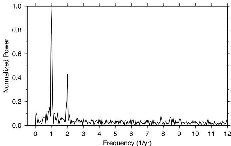
**Figure 8.** Periodogram of the beam power time series for the  $L_g$  noise from the Atlantic. The beam was steered due east with an apparent velocity of 4.0 km/s and the seismograms were bandpassed at 0.3–0.6 Hz with a 4-pole Butterworth filter. Prior to calculating the FFT the beam power values were converted to decibels relative to the median, the mean was removed, gaps were filled with linear interpolation, and the time series was padded with zeros to reach 8192 points.
