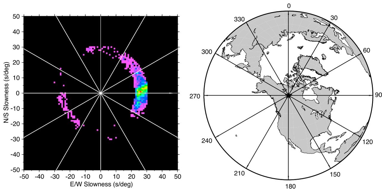
**Figure 6.** Comparison of f-k maxima from the broadband conventional procedure at a center frequency of 0.47 Hz (the middle right panel in Figure 5) with an orthographic map projection centered on YKA. This projection gives true angular directions (backazimuths) from the center that can be directly compared to directions in slowness space. In order to highlight the  $L_g$  energy, only f-k maxima with velocities between 3.6 and 5.0 km/s are shown.
