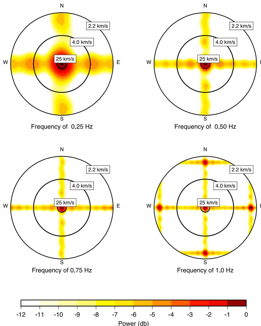
**Figure 2.** The slowness response of YKA to a vertically incident wave at frequencies of 0.25 Hz, 0.50 Hz, 0.75 Hz, and 1.0 Hz. An ideal array would give a single delta function at the origin. The outer radius of each panel is 50 s/deg (2.2 km/s), which is the same dimension used in the noise analysis. Note the poor resolution at low frequency (0.25 Hz) and the tiling at high frequency (1.0 Hz).
