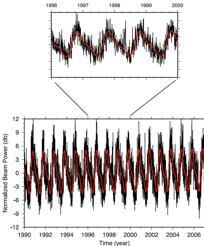
**Figure 9.** Power of a beam steered toward the  $L_g$  energy arriving from the east. The black curve represents the data, which are plotted as decibels relative to the median. The red curve is a least squares fit using the six-parameter model described in the text.
