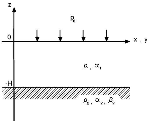
FIG. 3. Geometry of the geoacoustic model.
