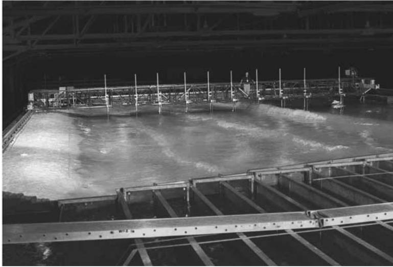
**Figure 1.** Movable bridge spanning the Large-Scale Sediment Transport Facility (LSTF).
