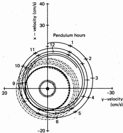
Figure 3: (After Jenkins [16].) Development in time (0 to 50 pendulum hours) of the mass transport velocity at depths of 0, 1, 2, 5, and 10 metres, after a monochromatic wave field of wave height 1.76 m propagates into the area of interest. Eddy viscosity =  $10^{-5} \text{ m}^2 \text{ s}^{-1}$ . (Reprinted from *Journal of Physical Oceanography*, © 1986 American Meteorological Society.)
