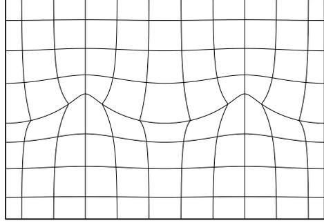
Figure 1: Example of a coordinate system, above and below a wave surface. In this particular case we have  $\mathbf{x} = (y_1 - ae^{-k|y_3|} \sin(ky_1 - \omega t), y_2, ae^{-k|y_3|} \cos(ky_1 - \omega t))$ . Above the interface, the coordinate system is isomorphic: below the interface  $J = 1 + O((ak)^2)$ .
