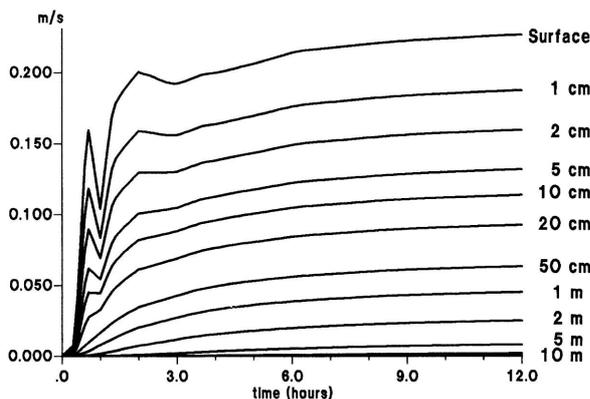
Figure 6: (After Jenkins [39].) The Stokes drift computed from the wave model results used in the coupled model runs for Fig. 5. (Reprinted from *Deutsche Hydrographische Zeitschrift*, © 1989 Bundesamt für Seeschifffahrt und Hydrographie.)
