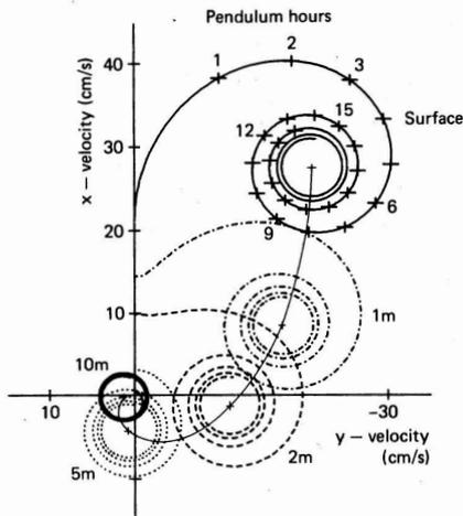
Figure 4: (After Jenkins [16].) Development in time of the mass transport velocity due to the same wave field as in Fig. 3. Eddy viscosity =  $10^{-5} \text{ m}^2 \text{ s}^{-1}$ . (Reprinted from *Journal of Physical Oceanography*, © 1986 American Meteorological Society.)
