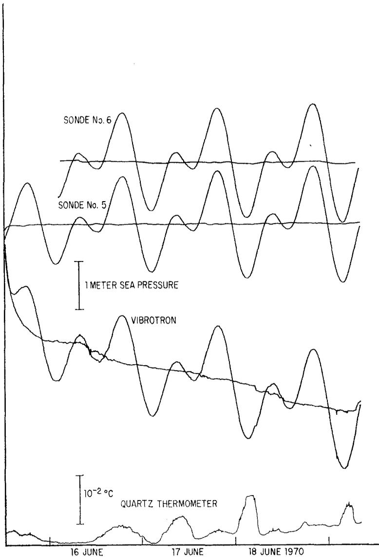
Fig. 3. San Clemente Sonde and Vibrotron pressure records, and a quartz-crystal temperature record. The residuals (after removal of the tides) are plotted with the record of each pressure sensor.
