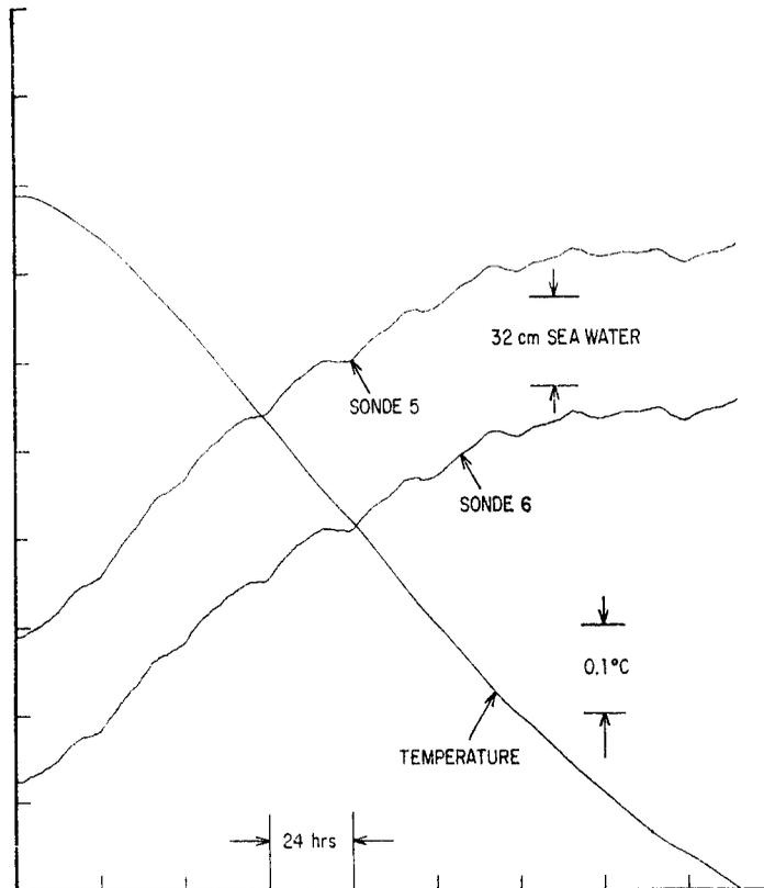
Fig. 1. Sonde pressure records and a quartz-crystal temperature record for a 210-hr noise test in 'flower bed'.
