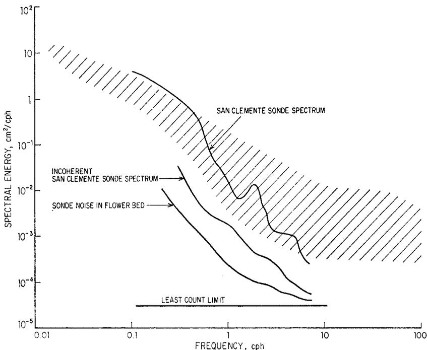
Fig. 2. The shaded band is based on 10 yr of measurements of background sea level oscillations. The San Clemente Sonde spectrum falls in the band and is more than 10 db above noise level.
