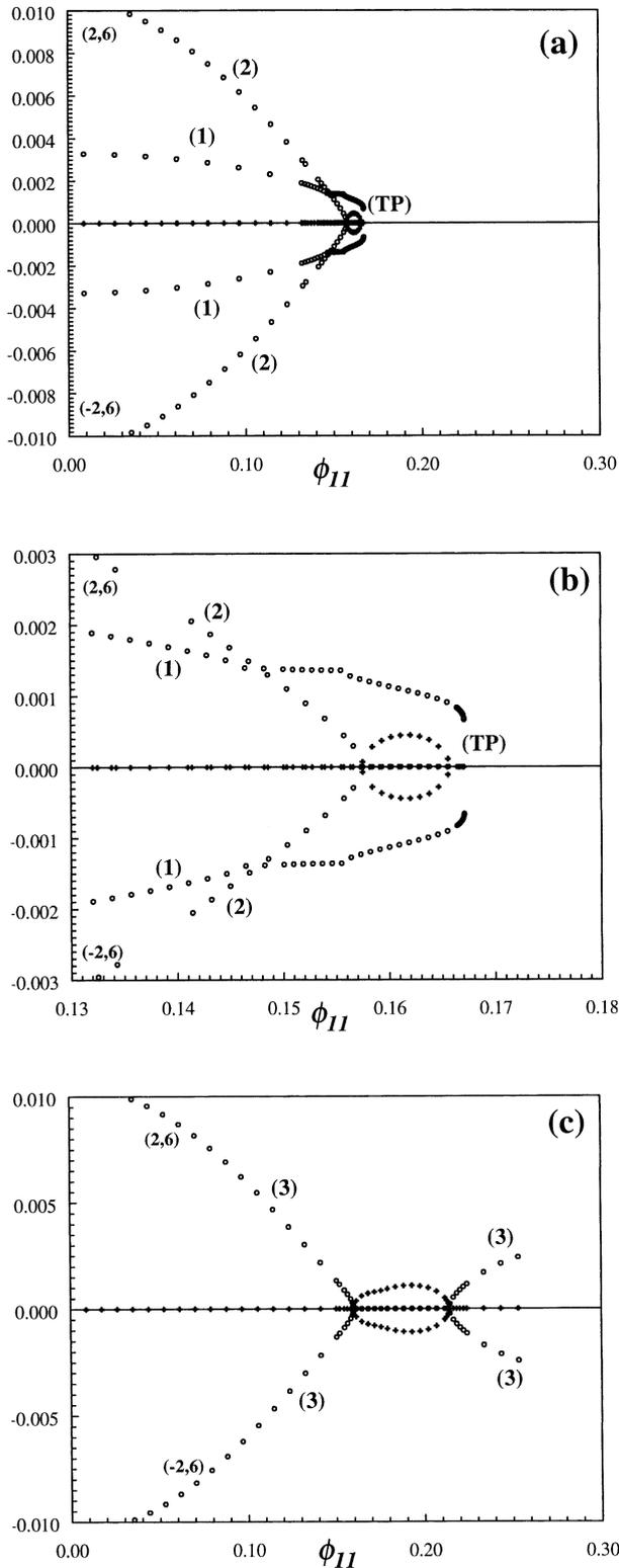
FIG. 3. Frequency  $[-\Re(\sigma_{\pm 2,6})]$  (open circles) and growth rate  $[-T(\sigma_{\pm 2,6})]$  (plus signs) as a function of coefficient  $\phi_{11}$  for depth  $d = 1$  and angle  $\theta = 66^\circ$ : (a) branches 1 and 2 including the TP area, (b) a magnification of (a), and (c) branch 3. See Fig. 2 for definition of the branches.
