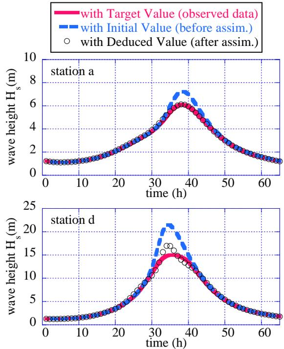
Fig.10 Comparison of computed wave heights at the station “a” and “d” where the examination was carried out for the case of the station “a” as the observation station.
