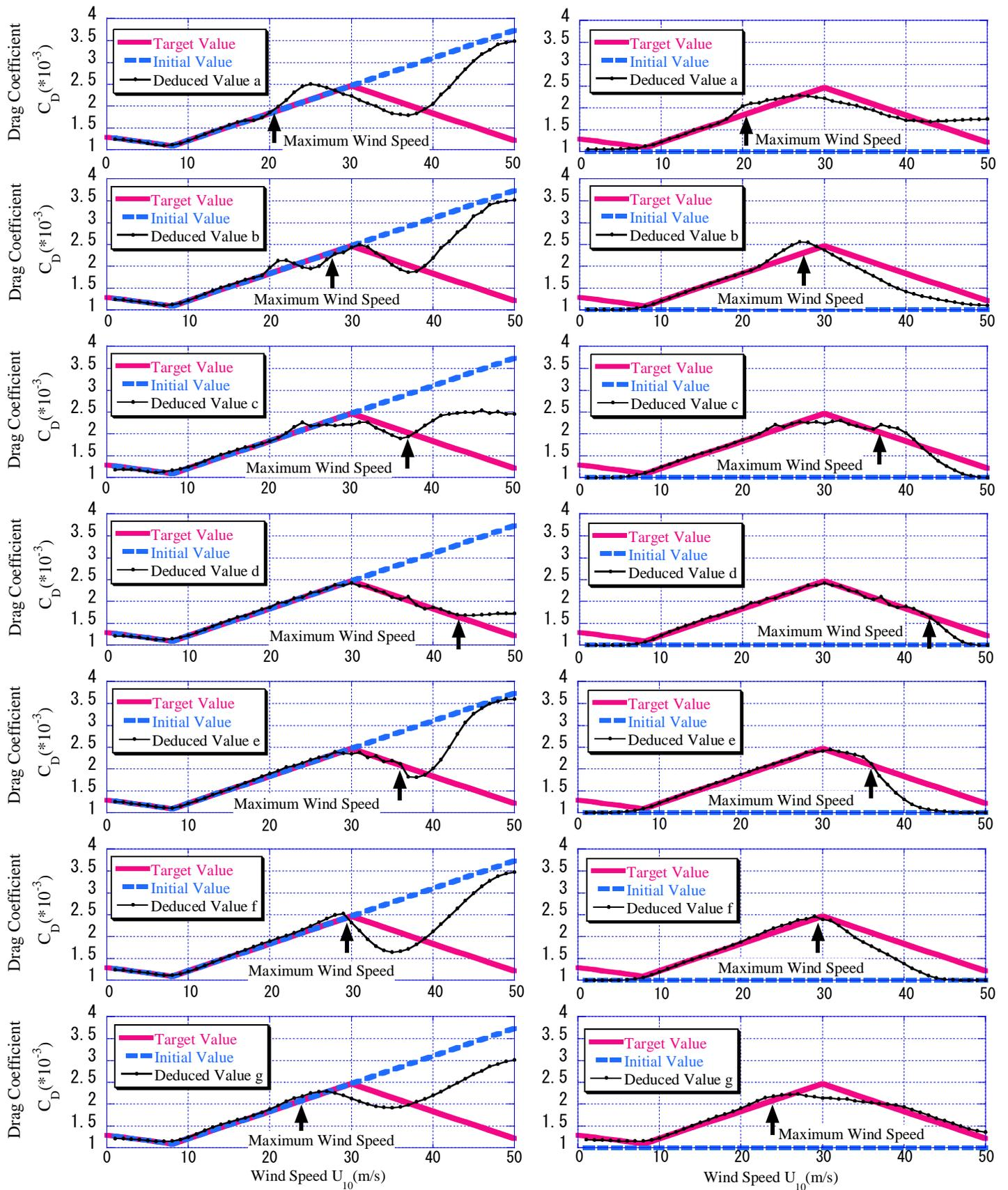
Fig.9 Deduced drag coefficients where distance from typhoon track is different
