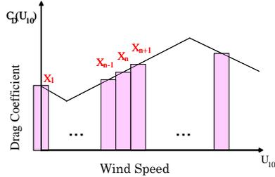
Fig.2 Drag coefficients assumed as a piecewise-constant function
