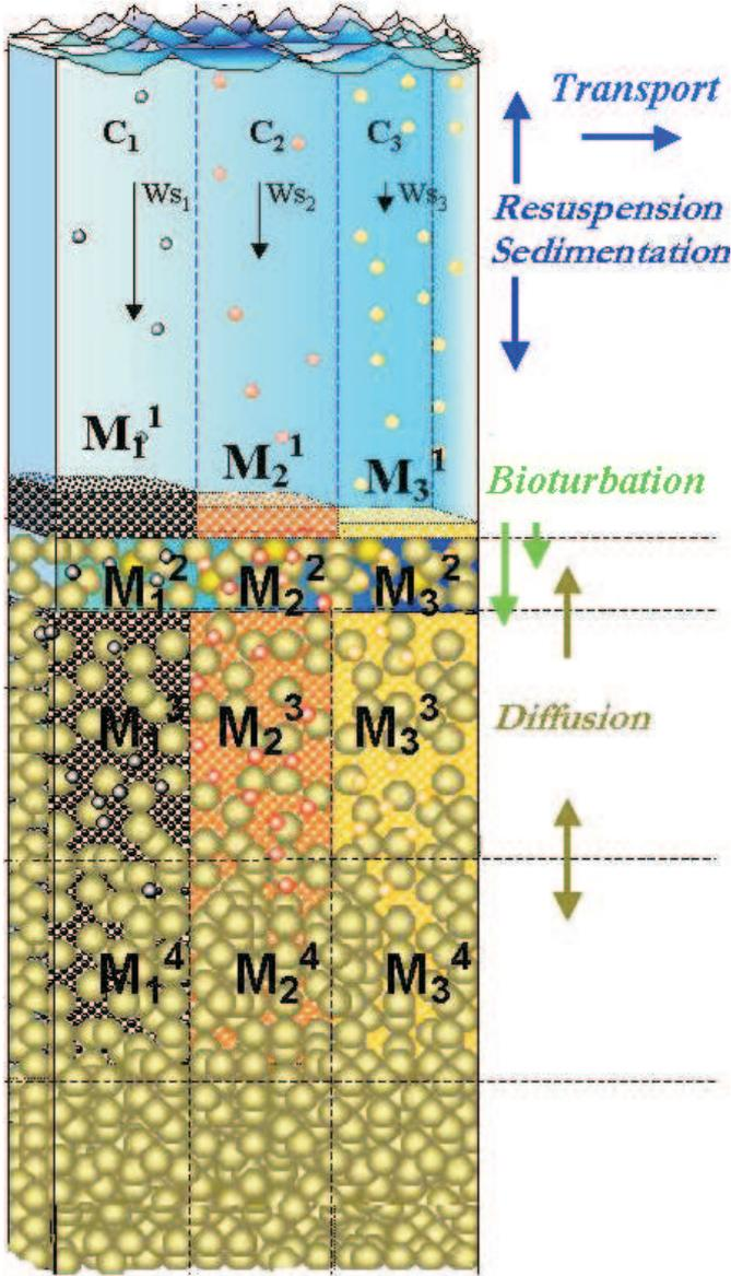
Fig. 2. Scheme of vertical exchange processes of SPM in the water column and bottom layers.
