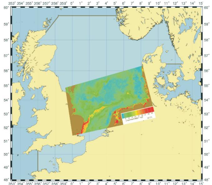
Fig. 1. SPM transport model area. Superimposed is the SPM surface concentration from a Coastal Zone Colour Scanner (CZCS) image.
