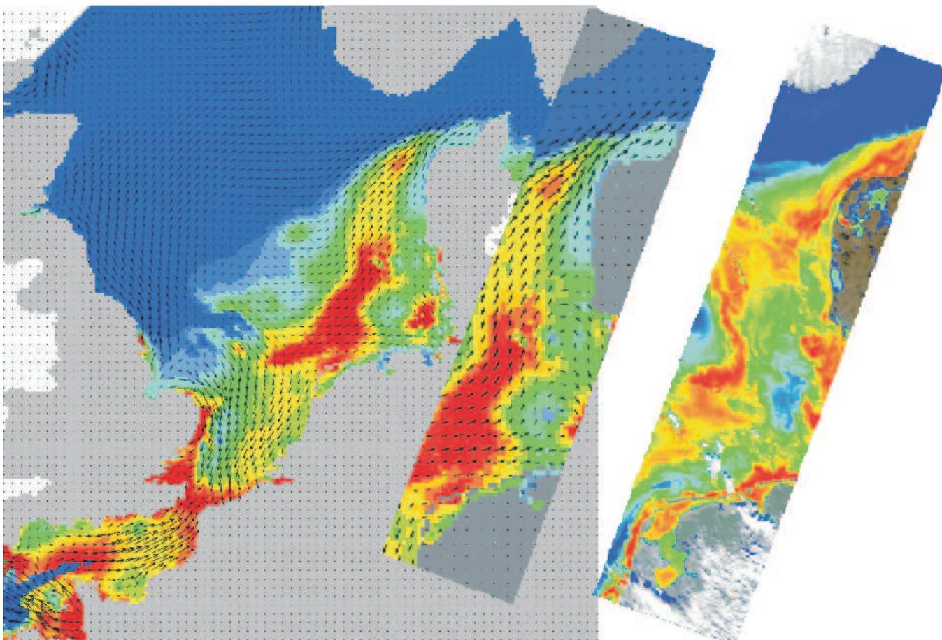
Fig. 3. Comparison of SPM surface concentration. Left: SPM model results. Right: results provided by the German space agency [6] as derived from a MOS image.
