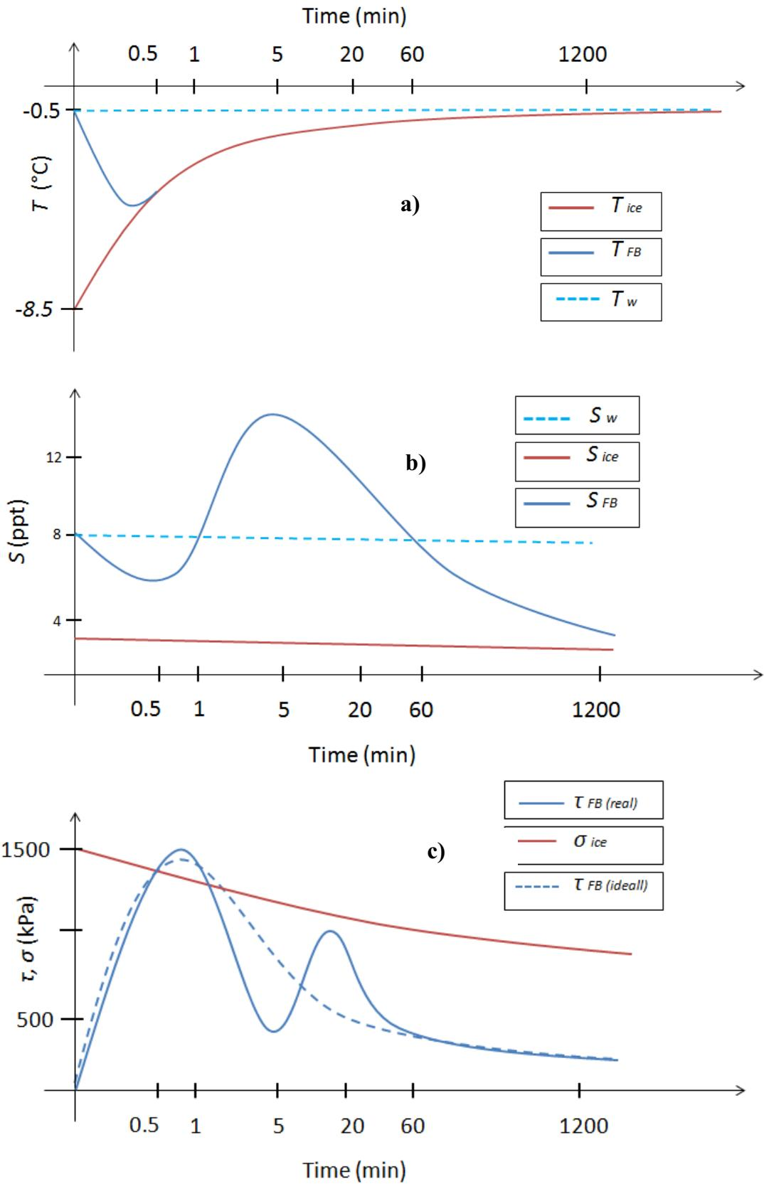
Figure 4. a) The ice temperature, b) the salinities and c) the peak stress in freeze-bond ( $\tau_{peak}$ ) vs. submersion time  $\Delta t$  for  $T_{i,0} = -8.5^{\circ}\text{C}$ .
