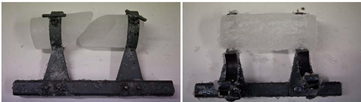
**Figure 2.** a) Sample about to be assembled in FIXIS, b) Sample right after the submersion in FIXIS.
