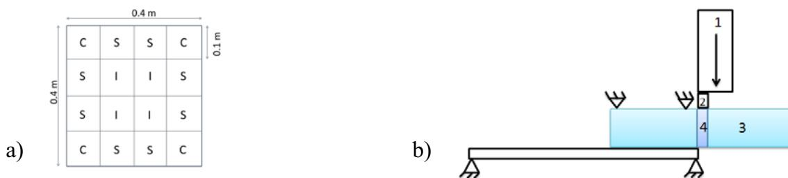
**Figure 1.** The big block experiments a) Sampling of Corner, Sides and Internal samples, b) The direct shear tests, 1 is the piston, 2 a wooden piece, 3 one of the original blocks and 4 the freeze-bond.
