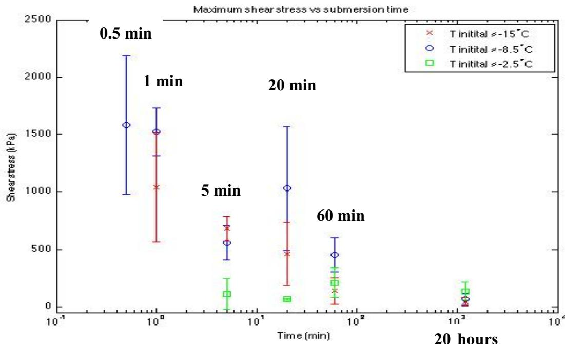
**Figure 3.** Peak shear stress ( $\tau_{peak}$ ) vs. submersion time ( $\Delta t$ ) for the three initial temperatures ( $T_{i,0}$ ) of  $-15^{\circ}\text{C}$ ,  $-8.5^{\circ}\text{C}$  and  $-2.5^{\circ}\text{C}$  and the six submersion times  $\Delta t = 0.5, 1, 5, 20, 60$  and  $1200$  minutes.
