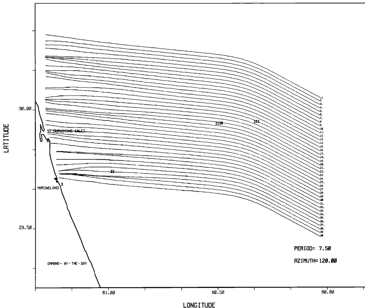
Fig. 10. Sample ray diagram illustrating wave-current interaction.
