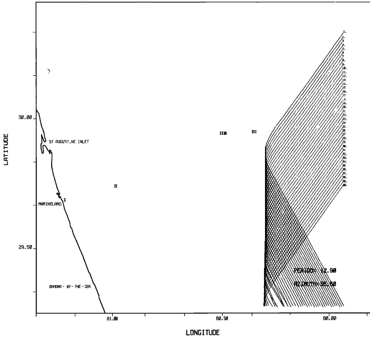
Fig. 9. Ray diagram of caustic pattern for incident angles where wave breaking and/or reflection occur. December 14, 1975, Marineland data.
