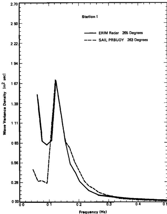
Fig. 7. Station 1: Radar spectra were derived from the geometry corrected Fourier transforms of the Erim SAR imagery. The pitch-and-roll buoy (PRBUOY) spectra is the average of nine 34-min spectra where the variance density of the radar spectrum was matched to the spectrum peak of the PRBUOY.
