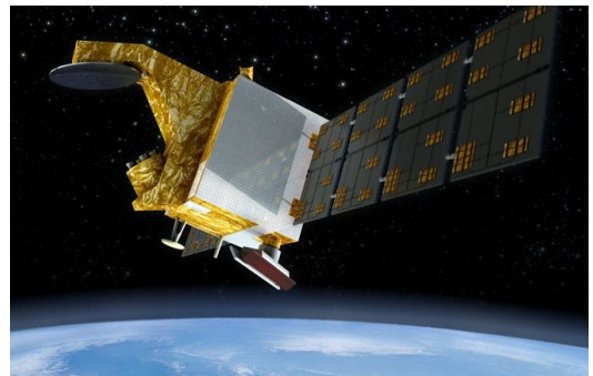
Figure 1. Artist view of the CFOSAT satellite. SWIM antenna is on the left (parabola pointing towards the surface and rotating plate with six feed horns) and SCATdual- antenna on the bottom right. Other antennas on Earth face are for TM/TC (X and S-bands). © CNES/ Gekko.
