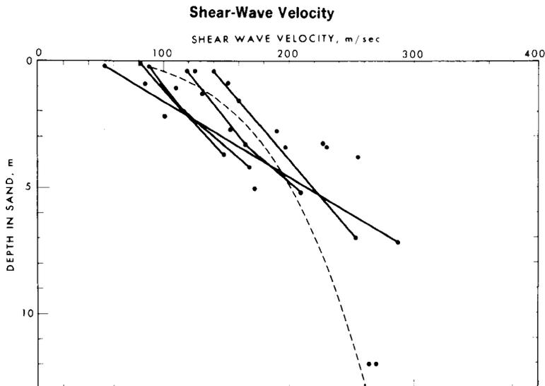
FIG. 1. Shear-wave velocity versus depth in selected water-saturated sands. Multiple measurements at the same site are connected by solid lines. The dashed line is the regression equation:  $V_s = 128(D)^{0.28}$ .
