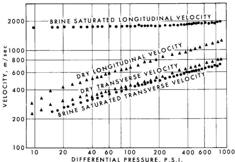
FIG. 3. Velocity of compressional (longitudinal) and shear (transverse) waves versus pressure in dry and brine-saturated (25 gm/liter NaCl) St. Peter fine sand (100-120 mesh, or 0.125-0.149 mm). By permission of the Shell Development Co. (personal communication, 1965); from Hamilton (1971a).
