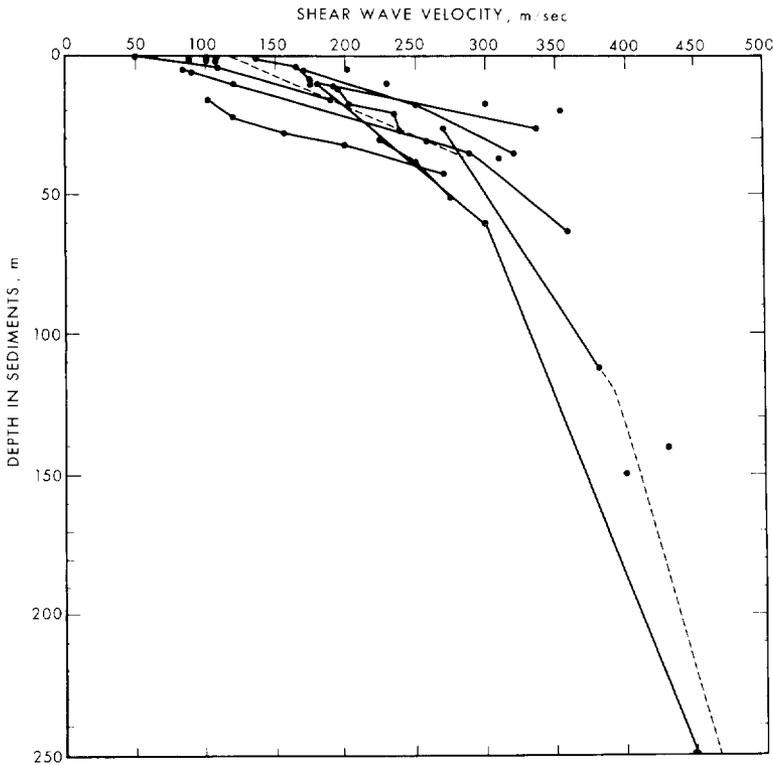
FIG. 2. Shear-wave velocity versus depth in selected water-saturated silt-clays and turbidites. Multiple measurements at the same site are connected by solid lines. The dashed lines are three regression equations. One measurement ( $V_s = 700\text{m/sec}$  at 650 m) is not shown.
