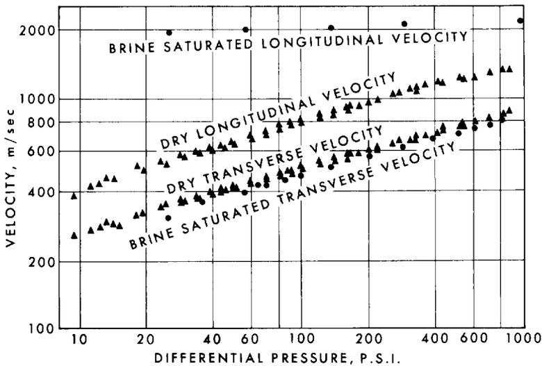
FIG. 4. Velocity of compressional (longitudinal) and shear (transverse) waves versus pressure in dry and brine-saturated (25 gm/liter NaCl) St. Peter coarse sand (20-30 mesh, or 0.59 to 0.84 mm). By permission of the Shell Development Co. (personal communication, 1965); from Hamilton (1971a).
