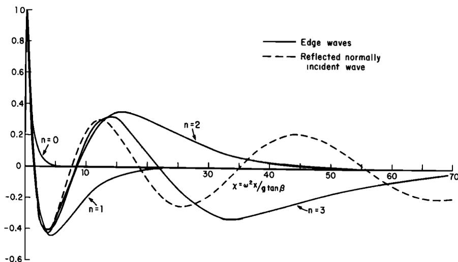
Fig. 1. Offshore dependence of profiles of Eckart-type edge waves of modes  $n = 0, 1, 2, 3$  and of normally incident reflected waves, in terms of the dimensionless variable  $\chi = \omega^2 x/g \tan \beta$ .
