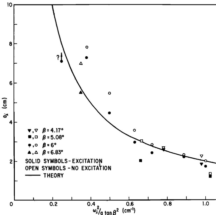
Fig. 4. Maximum incident wave amplitudes at the shoreline for zero mode subharmonic edge wave excitation (theory from (8)).
