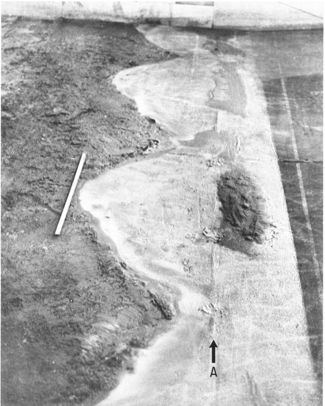
Fig. 8. Cusped morphologies produced by subharmonic edge waves; water has been drained below still level (marked 'A') to increase visibility. Black is sand, white is exposed concrete, and a meter stick is shown for scale.
