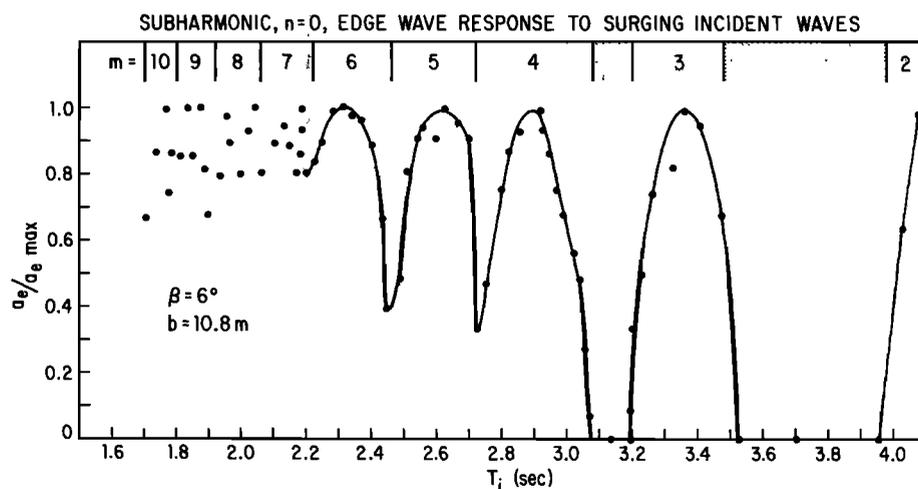
Fig. 7. Normalized edge wave response to surging incident waves of various periods. The vertical axis indicates the edge wave amplitude normalized by the maximum amplitude observed at a particular  $m$ . Synchronous edge waves were observed in the stippled region.
