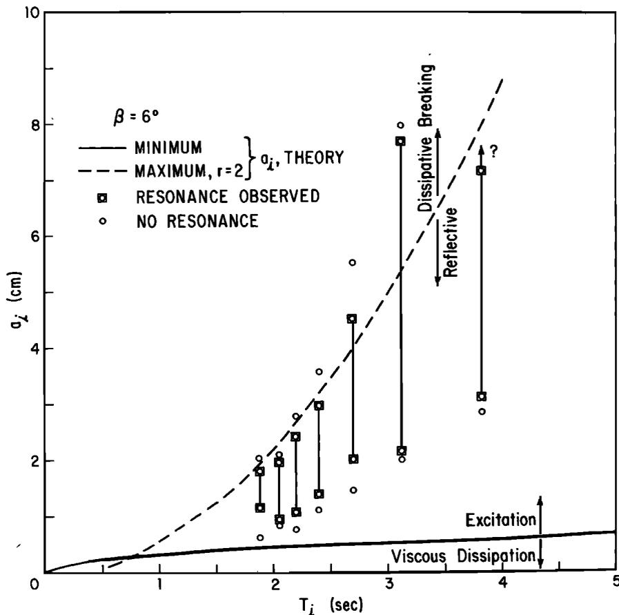
Fig. 3. Observed excitation of zero mode subharmonic edge waves as a function of incident wave period and amplitude. The dashed curve indicates the incident wave amplitude for transition from reflective to dissipative systems (equation (8)), and the solid curve indicates the amplitudes required to overcome viscous damping (equation (6)).
