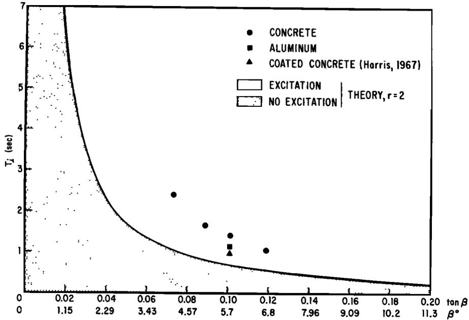
Fig. 5. Observed minimum incident wave periods (solid symbols) for  $n = 0$  subharmonic excitation on beaches of various slopes and smoothness (theory from (6) and (8)).
