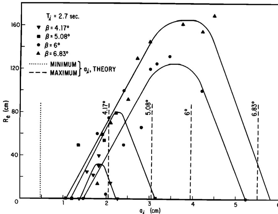
Fig. 6. Edge wave run-up amplitudes versus incident wave amplitudes for various beach slopes. The dashed lines are maximum incident wave amplitudes given by equation (8) and also correspond to the onset of plunging breakers.
