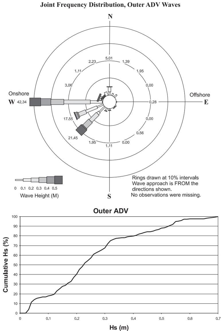
Fig. 3. Summary rose of breaking incident waves, and cumulative frequency plot of significant breaking wave height, 24 May–7 July 2002. Note the predominance of low wave heights, with 50% below 0.22 m. Wave data is from the outer ADV (RoseWorks software courtesy of UAI International).
