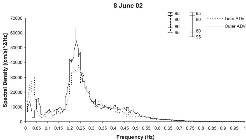
Fig. 7. Mean wave spectra, 13:30–18:30, 8 June 2002. Note the growth in infragravity energy under high wave energy conditions, with a distinct peak at 0.04 Hz on the inner ADV spectral record, and peaks at 0.06 Hz and 0.02 Hz on the outer ADV record.
