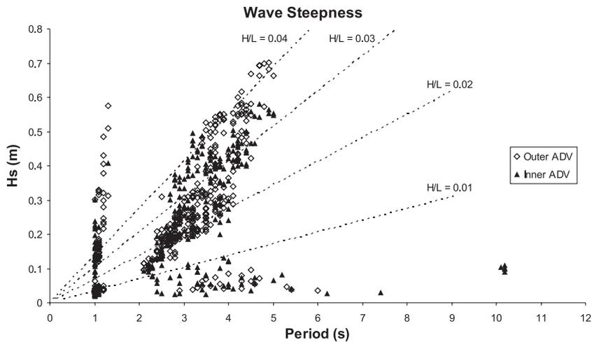
Fig. 4. Significant wave height and period from both instruments plotted against wave steepness isolines. Note the increase in wave steepness with increasing wave height.
