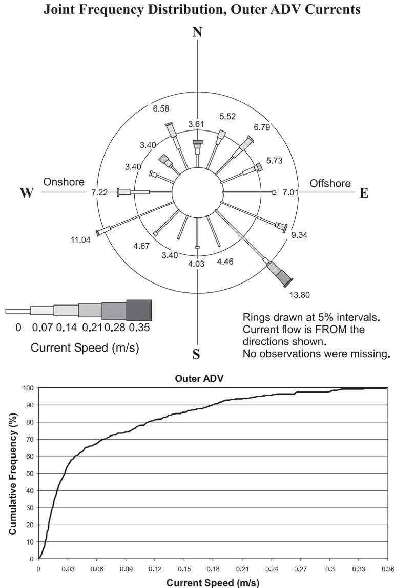
Fig. 5. Summary current rose and cumulative frequency plot of current speeds from the outer ADV, 30 April–7 July 2002. Note the wide dispersion of currents and the predominance of very low current speeds, with 60% below  $0.04 \text{ ms}^{-1}$ . The strong current flowing offshore from the southeast represents a rip current. (RoseWorks software courtesy of UAI International, Inc.).
