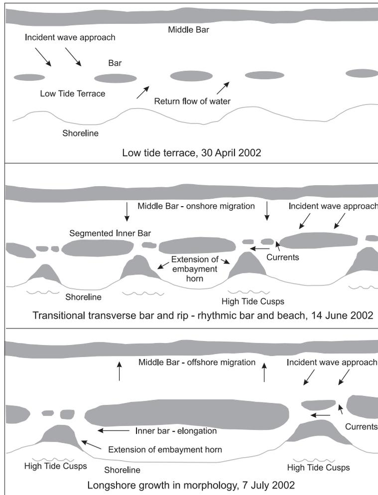
Fig. 9. Beach evolution from a low-tide terrace on 30 April 2002 to a transitional “transverse bar and rip-rhythmic bar and beach” on 7 July 2002. The change in beach state occurred during a high-energy event spanning 7 June–13 June 2002. Note the onshore movement of the middle bar. During a subsequent high-energy event (20–28 June 2002), there was an increase in the longshore scale of the beach morphology, but no further change in beach state. Note the offshore movement of the middle bar.
