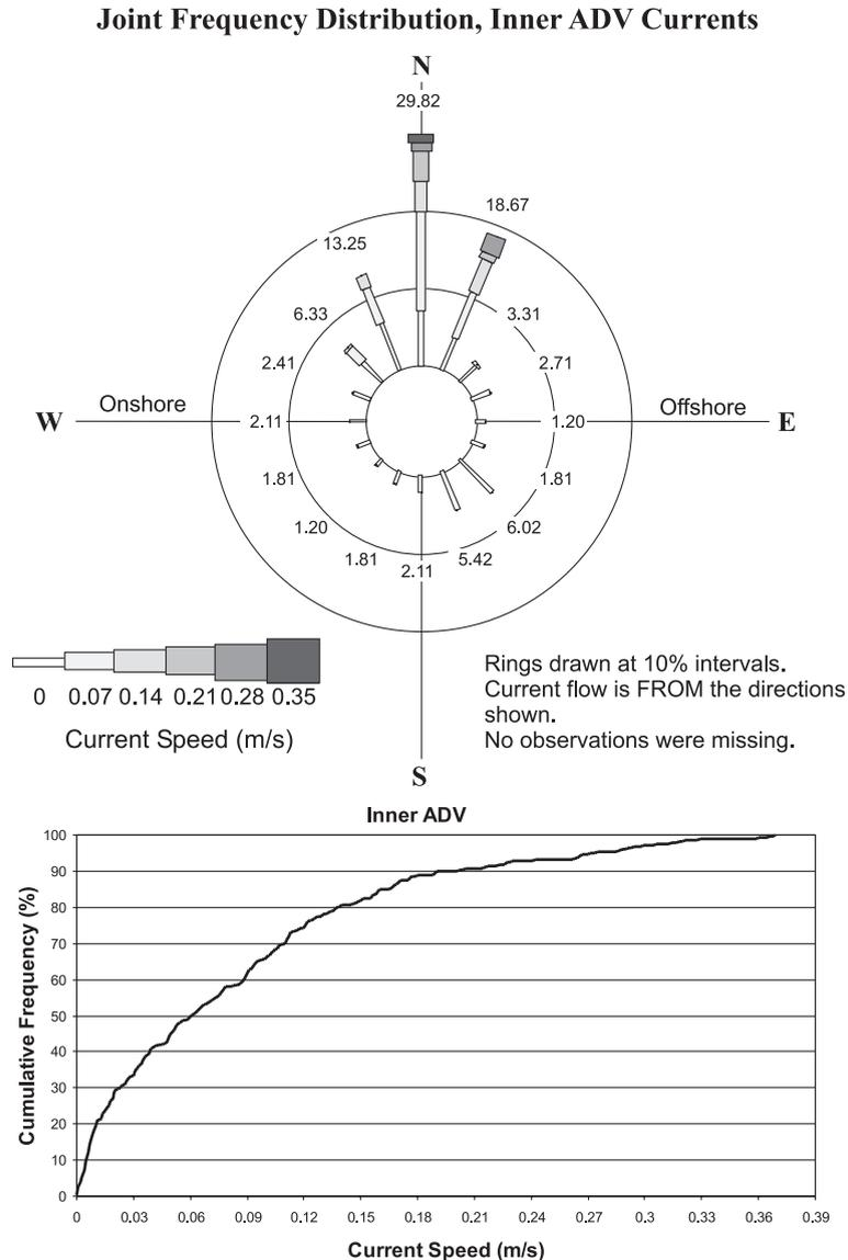
Fig. 6. Summary current rose and cumulative frequency plot of current speeds from the inner ADV, 30 April–7 July 2002. Note the striking dominance of a north to south longshore current, which attains a maximum speed of  $0.37 \text{ ms}^{-1}$  (RoseWorks software courtesy of UAI International).
