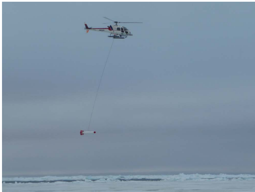
Figure 1. Sea ice thickness sensor with electromagnetic system and laser altimeter, hanging under a helicopter, and an automatic camera mounted on the helicopter (Photo: S. Gerland).
