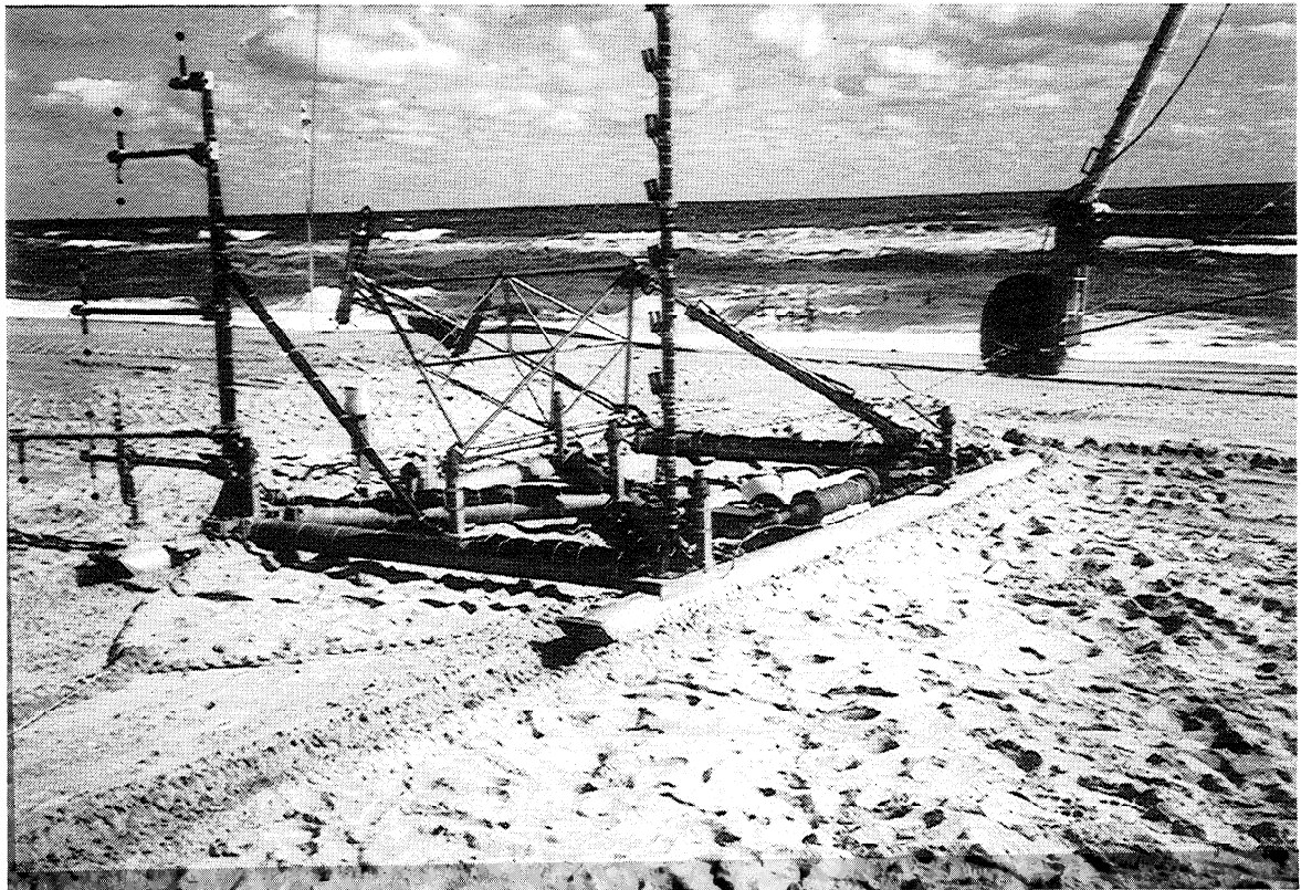
Figure 2. Photograph of the sled being pulled off the beach by the Coastal Research Amphibious Buggy (CRAB) (upper right) during DUCK94 experiment. Vertical array of electromagnetic current meters (ems) are mounted along the sled mast (center left).
