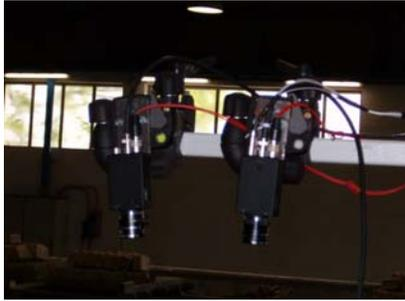
**Figure 1:** WASS physical set-up of two calibrated cameras.
