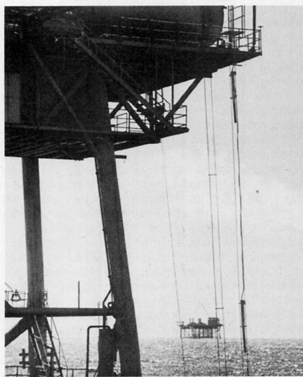
FIG. 1. Current meters being lowered into the water next to the wave staff at the Buccaneer A platform.
