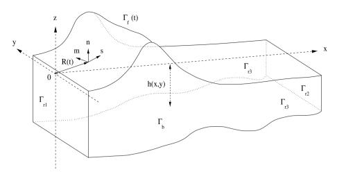
Fig. 1. Computational domain. The free surface  $\Gamma_{\rm f}(t)$  is defined at each time step by the position vector  $\mathbf{R}(t)$ . Lateral boundaries are denoted by  $\Gamma_{\rm r1}$ ,  $\Gamma_{\rm r2}$  and  $\Gamma_{\rm r3}$ . The bottom  $\Gamma_{\rm b}$  is defined by z=-h(x,y). Use is made of the Cartesian coordinate system (x,y,z) and of the local curvilinear coordinate system (x,y,z) and of the boundary.
