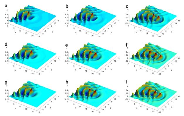
Fig. 12. Surface wave fields at breaking  $(t = t_{\rm BP})$ : d = 1 and  $\theta_{\rm max} = (a)$  40, (b) 45 and (c) 50; d = 2 and  $\theta_{\rm max} = (d)$  40, (e) 45 and (f) 50; d = 3 and  $\theta_{\rm max} = (g)$  40, (h) 45 and (i) 50. With:  $A^* = 0.315$  (6.3 m);  $\Omega = 1.282$ ; g = 1;  $N_{\theta} = 30$ .
