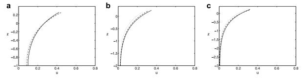
Fig. 17. Horizontal velocity u under the crest for a Stokes waves with the same height  $H_2$  and wavelength  $\lambda_2$  for d = (a) 1, (b) 2, (c) 3.
