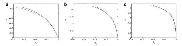
Fig. 19. Vertical acceleration  $a_z$  under the crest for an equivalent Stokes wave with the same height  $H_2$  and wavelength  $\lambda_2$  for d = (a) 1, (b) 2, (c) 3.
