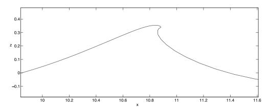
Fig. 11. Close-up of the overturning crest at y = 0 and t = 6.89T for cases of Figs. 4 and 7.
