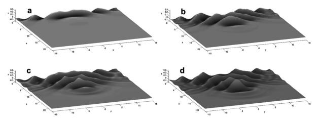
Fig. 3. Free surface evolution at: (a) t = 3.11T, (b) t = 4.74T, (c) t = 6.20T, (d) t = 6.89T. In the last figure, the focused wave is starting to overturn, with its crest located at x = 211 m (or 10.55d).
