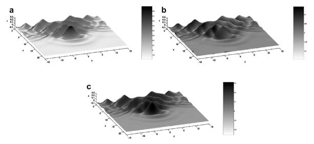
Fig. 10. Same case as Fig. 3d. Velocity field components on the free surface at t = 6.89T (breaking time): (a) u, (b) v, (c) w.
