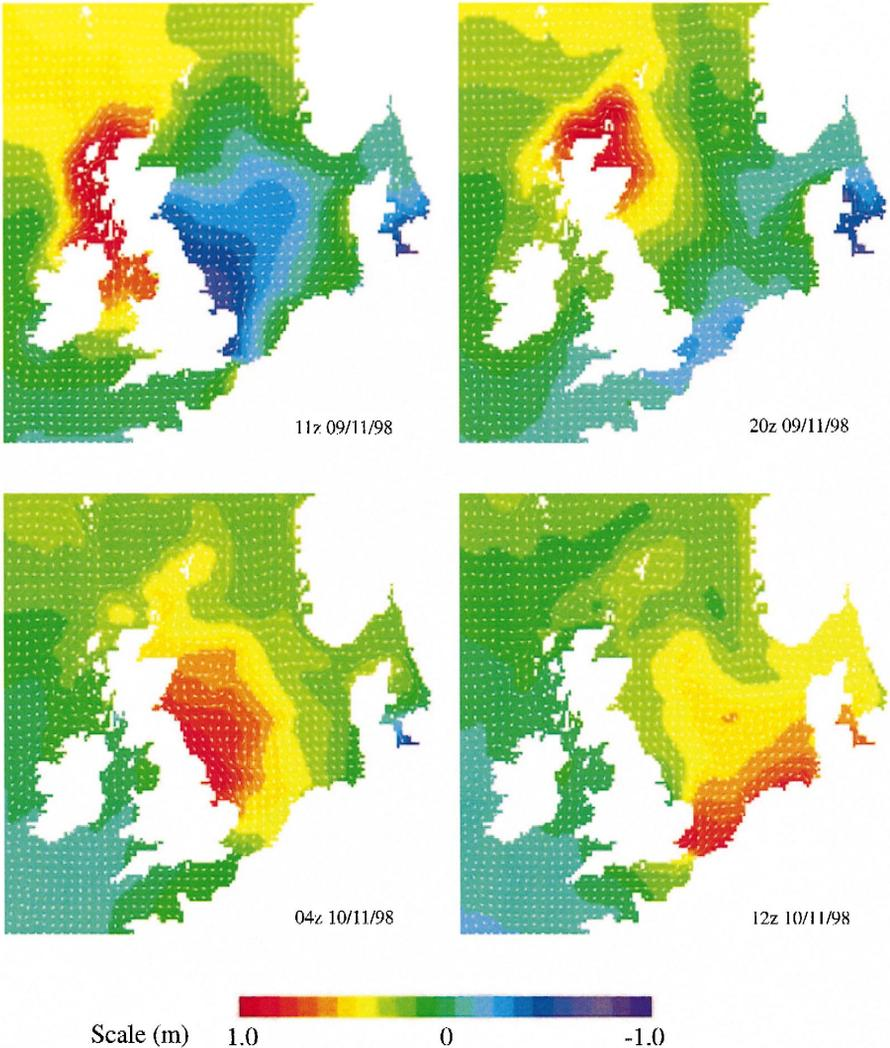
Fig. 9. A typical external surge event from the UK operational storm surge model archive, showing surge generation west of Scotland, followed by propagation around the north of Scotland and southwards along the east coast of England into the southern bight of the North Sea.
