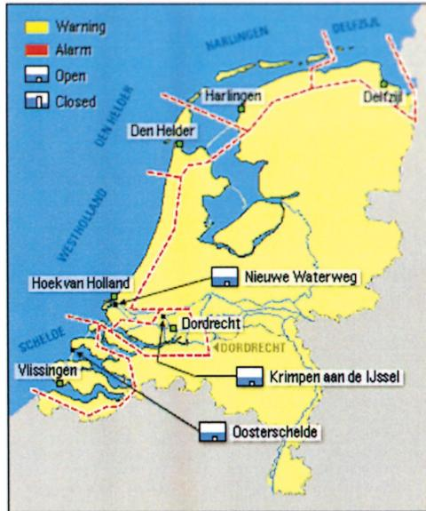
Fig. 8. Status of coastal sectors and flood barriers from the Dutch Storm Surge Warning Service (SVSD) web page, <http://www.waterland.net/>.
