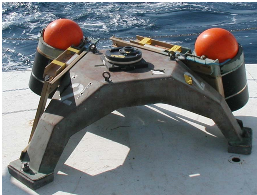
Figure 4. Sea spider tripod with a pressure sensor in the center and dual acoustic release recovering systems.
