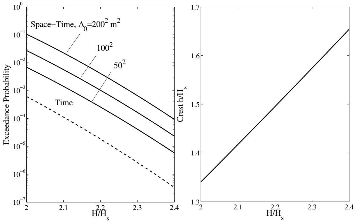
FIG. 7. ERA-interim reanalysis at the time of maximum development of the Draupner storm (Jan 2st 1995 UTC 00) at the platform site (58.2 N, 2.5 E). Left: space-time probability  $P_{ST}(H/H_s; A_0, D)$  for  $A_0 = 50^2, 100^2, 200^2 m^2$  and corresponding time probability  $P_T(H/H_s; D)$  as a function of  $H/H_s$  and  $D = 3$  hours. Right: exceeded second order nonlinear crest height  $h/H_s$  as a function of  $H/H_s$ .
