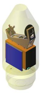
Figure 5.52. Accommodation of SKIM in the Vega-C fairing on top of short VESPA-C, Concept A (left) and Concept B (right).
