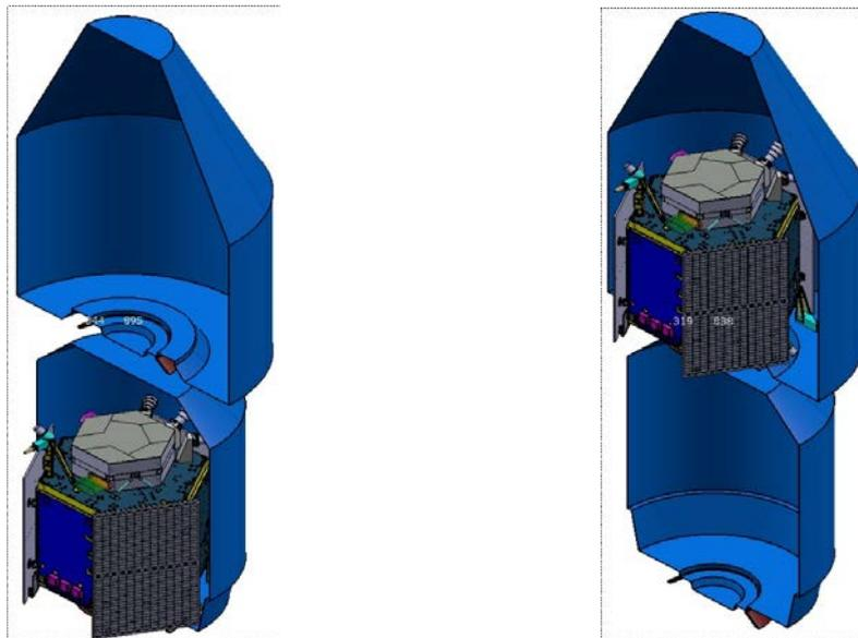
Figure 5.43 Concept A accommodation in the Vega-C fairing, inside (left) and on top (right) of the VESPA-long.
