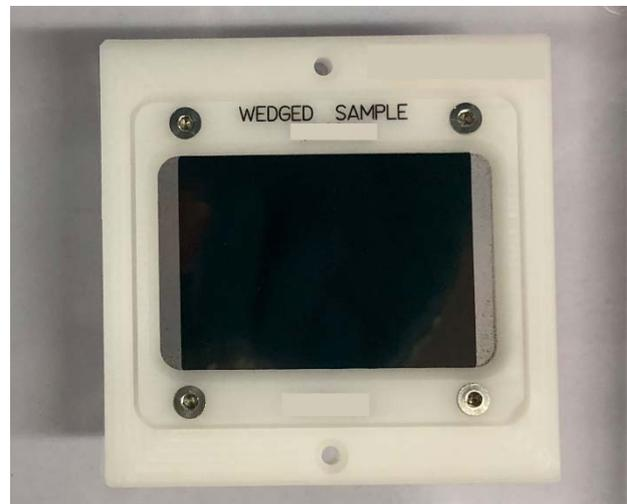
Figure 5.19 FSI interferometer full size wedged diamond beamsplitter breadboard uncoated (Left) and after Germanium coating (Right) - Concept B
