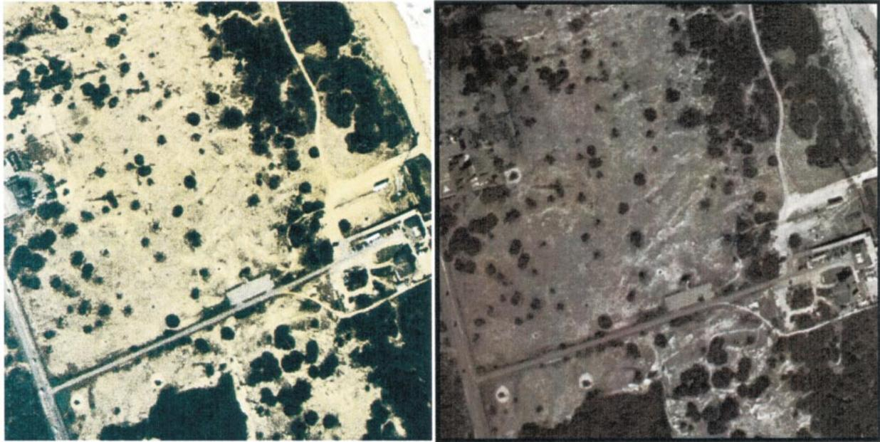
FIG. 4. Comparison of (a) an aerial survey photo of the area around the Army Corps of FRF in Duck, NC, and (b) an AROSS image after mapping to geographic coordinates on a uniform rectilinear grid. These images are about 1 km across.
