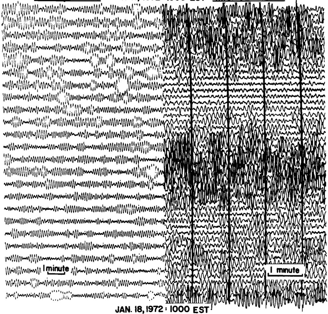
Fig. 1. Vertical portions of 24-hour drum records of microseisms and microbaroms; the microbaroms show strong semidiurnal amplitude variations, whereas microseisms are essentially unchanged in amplitude. Time scale of the seismogram, whose drum rotation rate is 24/day, is one-half the scale of the microbarogram having 48 rotations per day.
