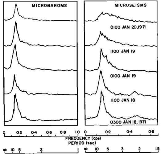
Fig. 5. Comparison of simultaneous amplitude spectra of microseisms and microbaroms for January 18-20, 1971.
