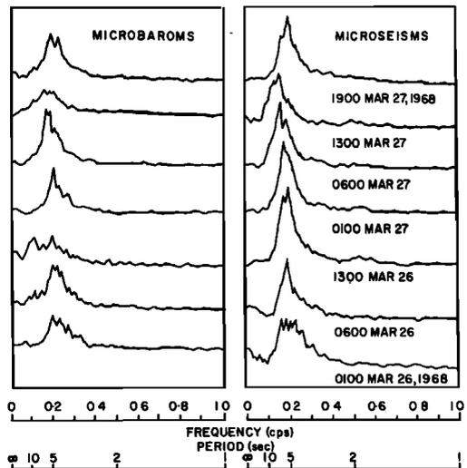
Fig. 2a. Simultaneous amplitude spectra of microseisms and microbaroms at seven distinct intervals during March 26–27, 1968. Each spectrum was taken over a continuous interval of 20 min duration. All times are GMT.
