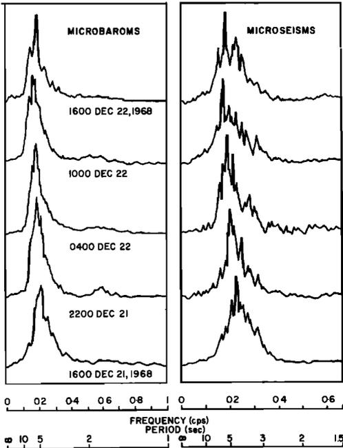
Fig. 4. Comparison of simultaneous amplitude spectra of microseisms and microbaroms for December 21-22, 1968.
