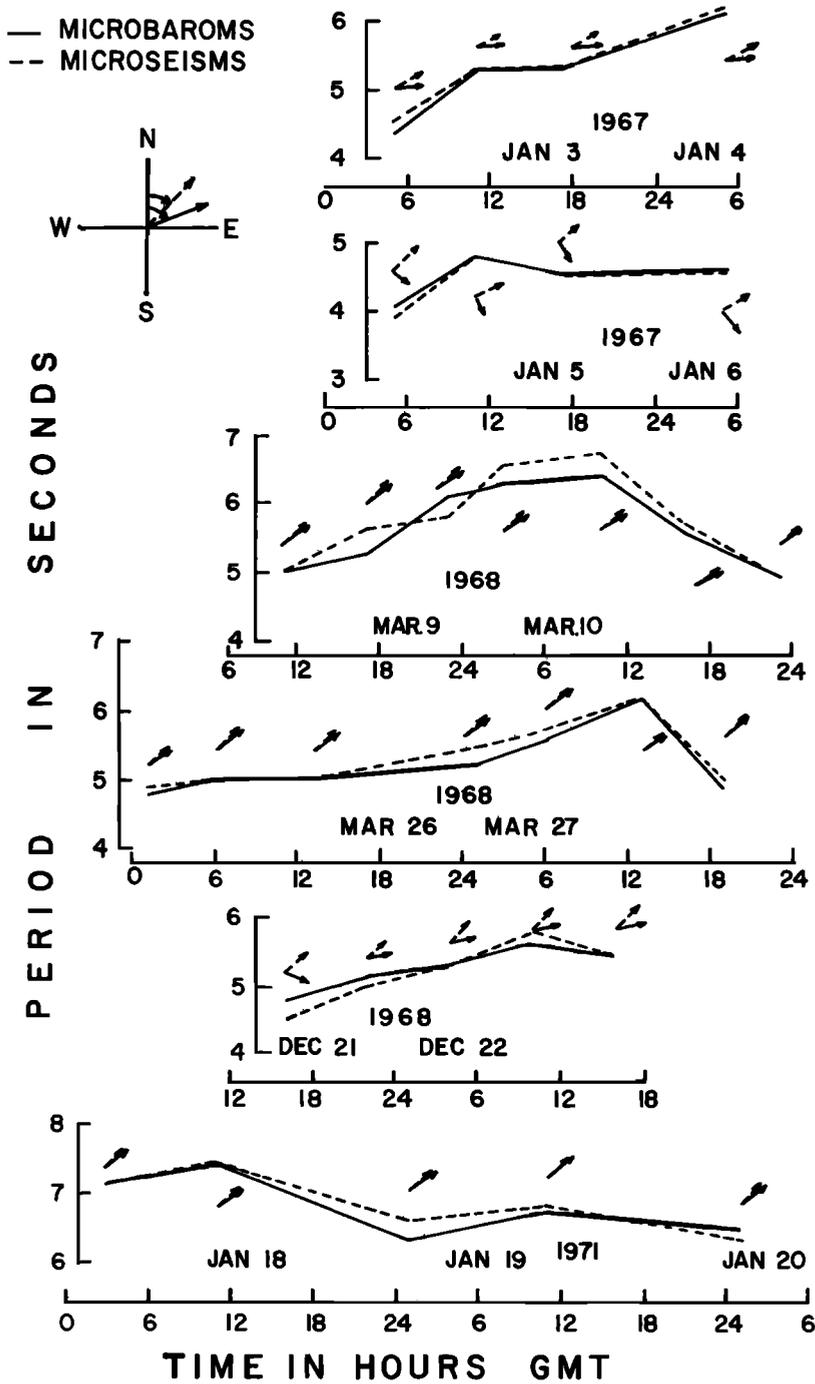
Fig. 6. Time series of simultaneous spectra of microseisms and microbaroms for a number of cases, together with arrows indicating source directions at the time of each computation.
