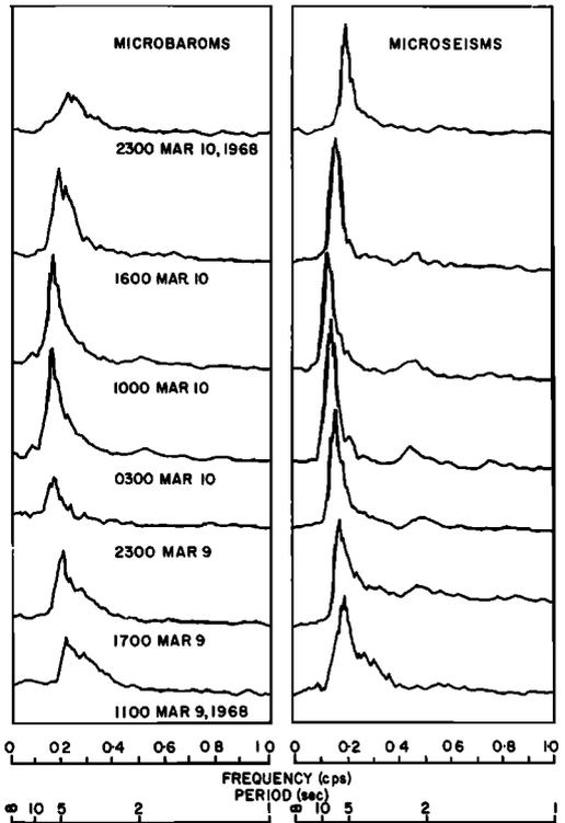
Fig. 3. Comparison of simultaneous microseism and microbarom amplitude spectra for March 9 and 10, 1968.
