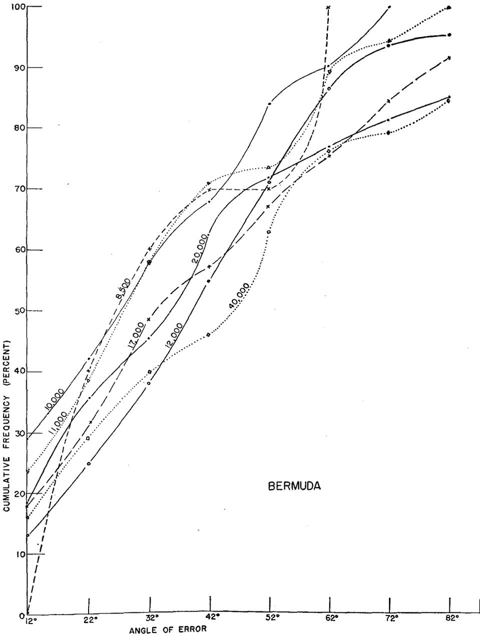
Fig. 5. Graph of cumulative frequency of angles of error associated with velocities at Bermuda. Curves show velocity in feet per second.
