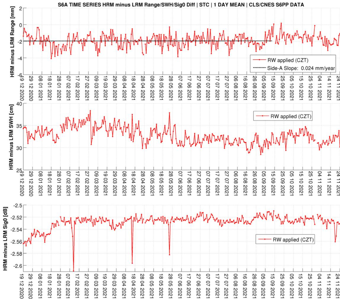
Fig. 42. Time series of the difference between the HRM and LRM for range (top), SWH (middle), sigma0 (bottom) for the STC latency. The range walk (via CZT-based beam-forming) is applied on HRM side and both HRM and LRM are retracked with the numerical retracker using the in-flight PTR interface.
