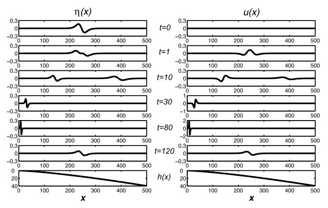
**Figure 3.** (left) Water displacement and (right) velocity for initial disturbance (27). The bottom profile is shown at the bottom.
