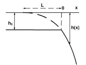
Figure 7. The geometry of a shallow coastal area and a convex slope.
