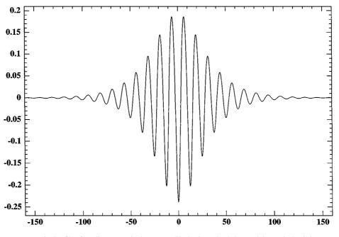
*Figure 3* Profile of a solitary wave in deep water. The horizontal axis is X and the vertical axis is  $\eta$ .
