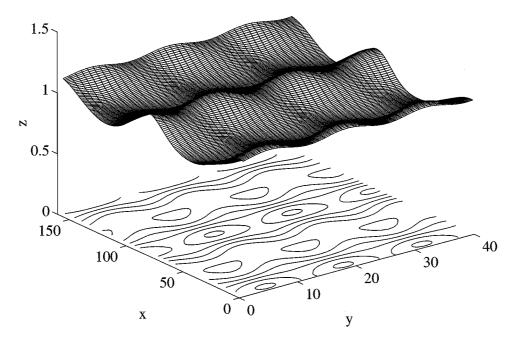
*Figure 7* 3D wave pattern that has evolved from a uniform Stokes wave train ( $\epsilon = 0.23$ ) by instability of class II (m = 1) with  $p = \frac{1}{2}$  and  $q = \frac{3}{2}$ . The waves are propagating from right to left. The horseshoe patterns are in their phase of growth and have their wave fronts oriented forward. Drawing by C Skandrani (1997).
