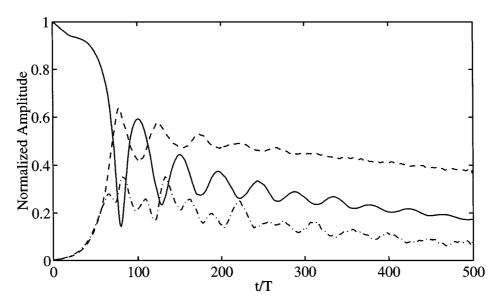
*Figure 6* Time histories of the amplitude of the fundamental, subharmonic, and superharmonic modes  $(p = \frac{1}{3})$  for an evolving perturbed train of Stokes waves of initial steepness  $\epsilon = 0.20$ , wavelength L = 10 cm, and fundamental period *T*.
