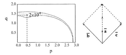
*Figure 8* Selection of the dominant triad. Instability region for the Stokes wave of steepness  $\epsilon = 0.3$  (the dot labels the point of maximum instability) and the dominant symmetric resonant triad in **k**-space.
