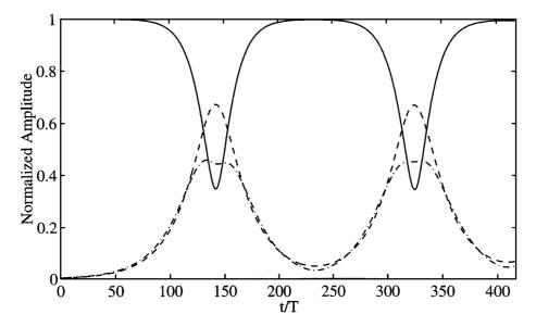
*Figure 5* Time histories of the amplitude of the fundamental, subharmonic, and superharmonic modes  $(p = \frac{2}{9})$  for an evolving perturbed Stokes wave of initial steepness  $\epsilon = 0.13$  and fundamental period *T*.
