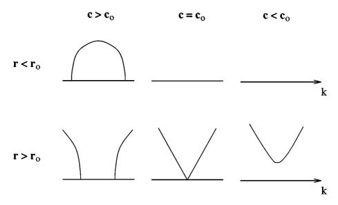
*Figure 2* Bifurcation of periodic traveling waves near the critical point  $(k_o, c_o)$  when  $r \neq r_o$ . The case  $c > c_o$  was explained in Figure 1. For  $r < r_o$ , there are no periodic solutions with  $c < c_o$ . For  $r > r_o$ , the branches of periodic solutions coalesce at  $c = c_o$  and become a detached branch for  $c < c_o$ . These new periodic solutions exist only at finite amplitude.
