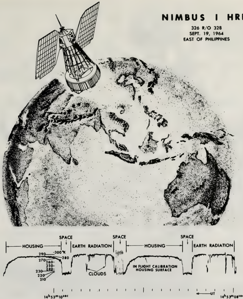
Figure 22.1 Portion of an HRIR analog record of NIMBUS I. In the example, the mirror made two complete revolutions, scanning the effective radiation temperature of space and the radiometer housing as well as the earth. The space and radiometer housing data are useful in positioning the satellite and calibrating the radiometer (after LaViolette and Chabot, 1968).
