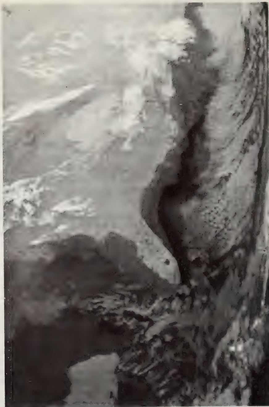
Figure 22.4 ITOS-1 scanning radiometer IR picture over the East coast of the United States, February 15, 1971, orbit No. 4853. The northern boundary of the Gulf Stream is clearly visible. Temperature gradients over the Bahama Banks and in the Gulf of Mexico are also visible (after Watson, 1971).
