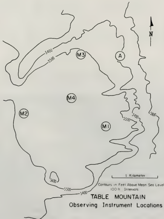
Figure 7.9 Location of the observing instruments on Table Mountain. The circles marked M1, M2, M3, and M4 indicate the positions of the microbarographs, and the circle marked A represents the position of the acoustic sounder. The entire system is located just east of the foothills of the Rocky Mountains (from Hooke et al., 1971).
