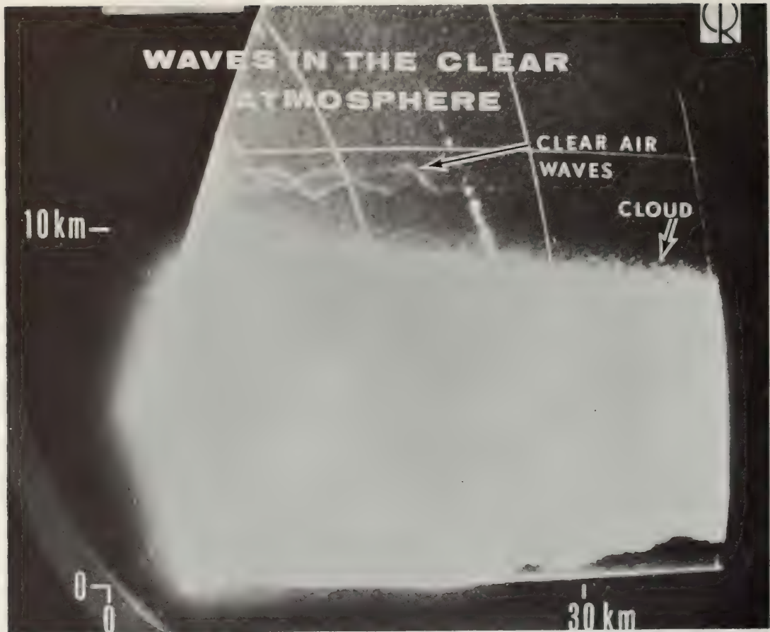
Figure 14.14 Photograph of RHI at wavelength of 10.7-cm, 1509 EST, 7 Feb 1968 at Wallops Island, Virginia, azimuth 270 deg. Cloud and precipitation extend from the surface to about 10 km. The unusual clear-air echo structure of apparently crossing waves out of phase occurs at 11.3 km, the height of the tropopause. This is a good example of the "braided" structure illustrated in (F14.12) (from Hardy et al., 1969).
