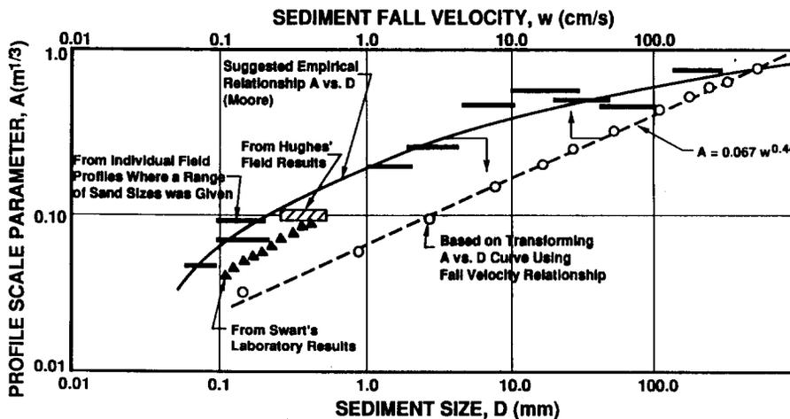
Fig. 2. Beach profile factor,  $A$ , vs. sediment diameter  $D$ , and fall velocity,  $w$ , in relationship  $h = Ax^{2/3}$  (Dean, 1987; modified from Moore, 1982).
