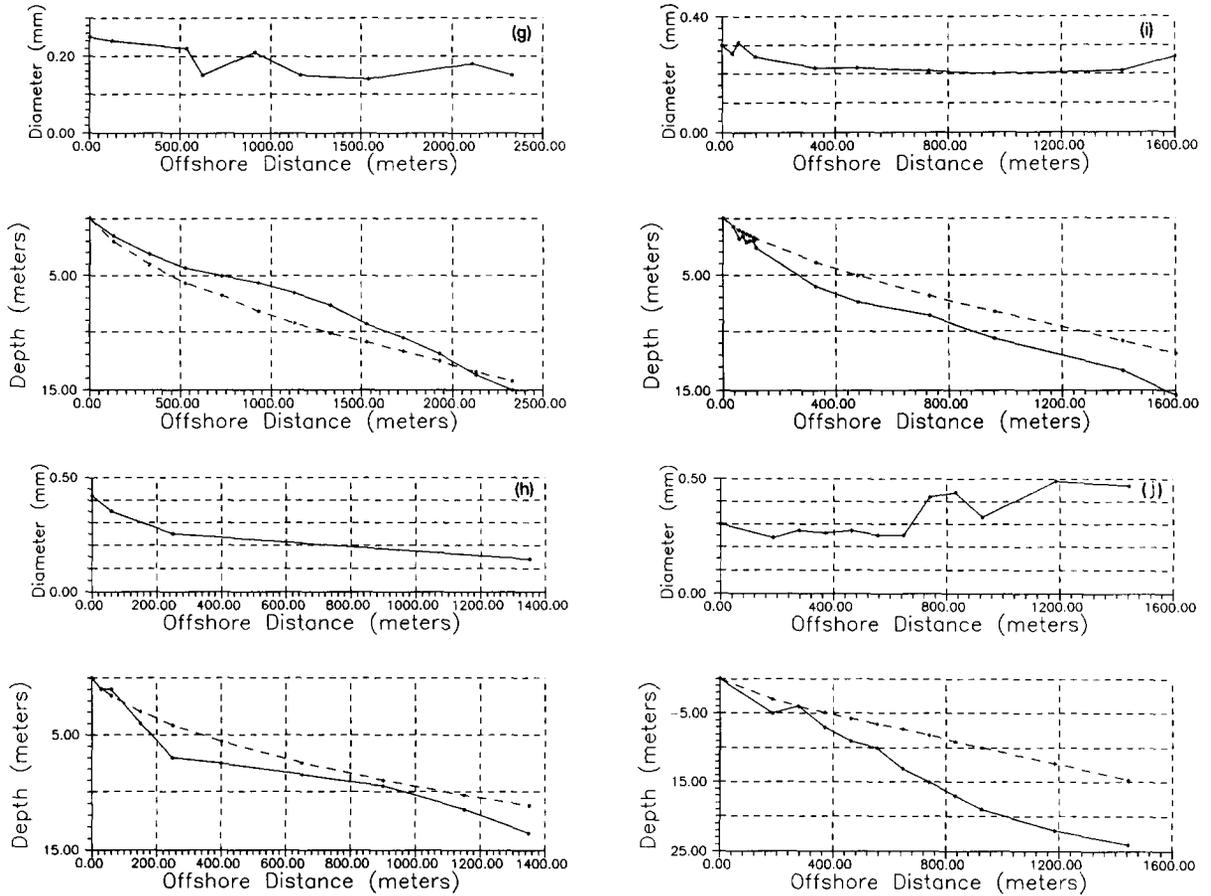
Fig. 7. Measured sediment sizes and comparison of measured and predicted profiles. Measured = Solid Line, Predicted = Dashed Line. (a) Ohiwa Beach;  $BSL=0.048$ . (b) Ohope Beach;  $BSL=0.063$ . (c) Piripai Beach;  $BSL=0.064$ . (d) Matata Beach;  $BSL=0.073$ . (e) Papamoa Beach;  $BSL=0.055$ . (f) Mt. Maunganui Beach;  $BSL=0.077$ . (g) Waihi Beach;  $BSL=0.038$ . (h) Whiritoa Beach South;  $BSL=0.072$ . (i) Omaha Beach;  $BSL=0.031$ . (j) Pakiri Beach;  $BSL=0.056$ .
