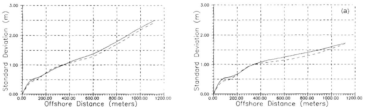
Fig. 9. Comparisons of running standard deviations between measured profiles and their average at each point (solid line) and the measured and calculated profiles at each point (dashed line). Total of ten profiles. (a) Total of nine profiles.
