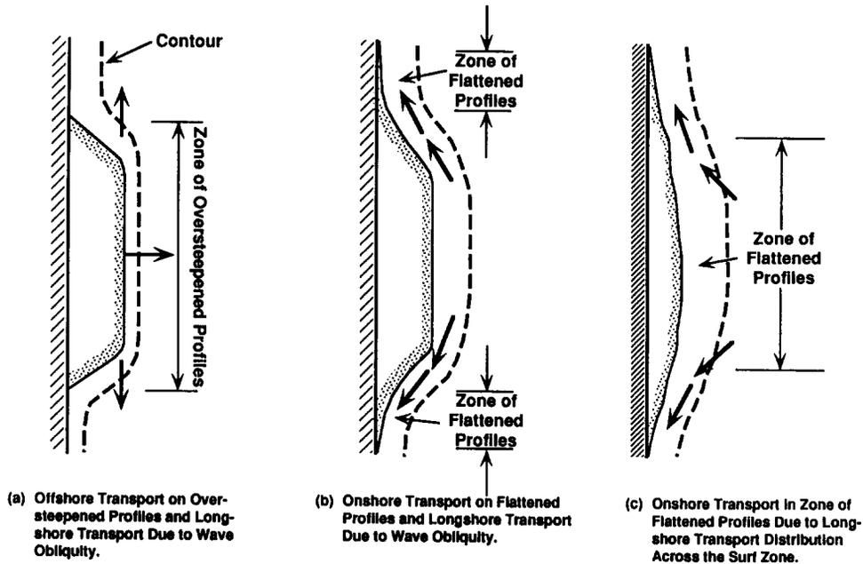
Fig. 5. Three phases of observed sediment transport in vicinity of nourished projects. *Note:* cross contour transport due to profile disequilibrium.
