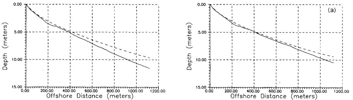
Fig. 8. Comparison of average measured profile (solid line) and predicted profile (dashed line). Total of ten profiles. (a) Total of nine profiles (without Pakiri profile).
