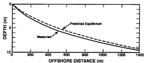
Fig. 4. Illustration of measured profile in equilibrium over the depth range,  $5 \text{ m} < h < 9 \text{ m}$ , even though profiles are displaced horizontally.
