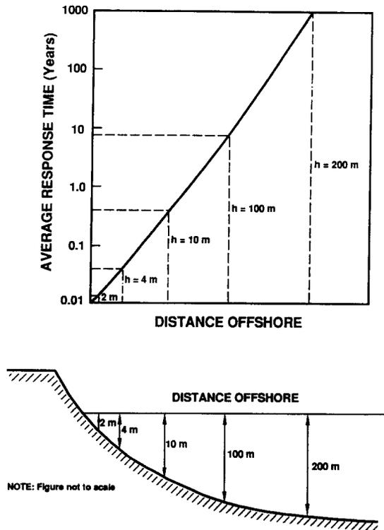
Fig. 1. Concept of increasing response times for greater water depths.
