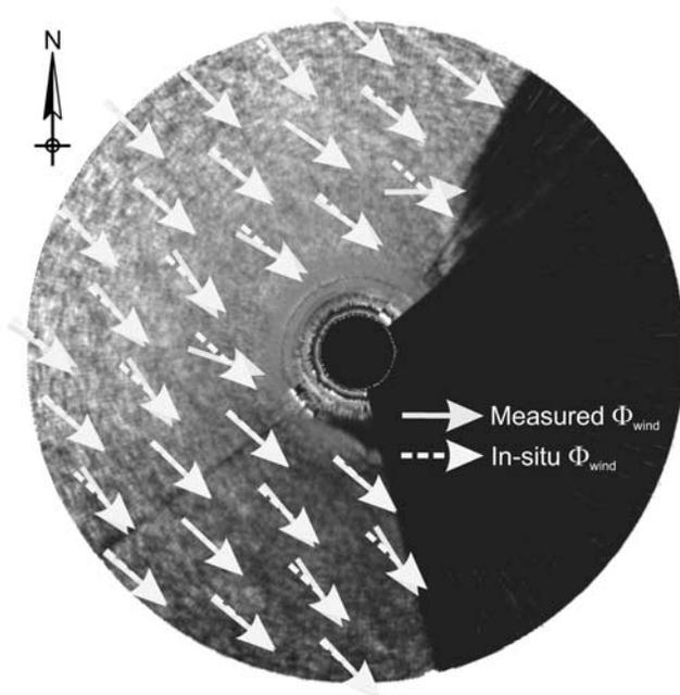
**Figure 5.** Mean RCS of a radar-image sequence from Ekofisk 2/4 k on April 15, 2001. The wind speed was  $8 \text{ m s}^{-1}$ , and the measured wind direction at 74 m height (dashed arrows) was  $335^\circ$ . Superimposed are solid arrows giving the retrieved local wind direction at the ocean surface.
