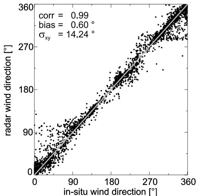
**Figure 6.** Scatterplot of in situ wind directions versus radar-derived wind directions.
