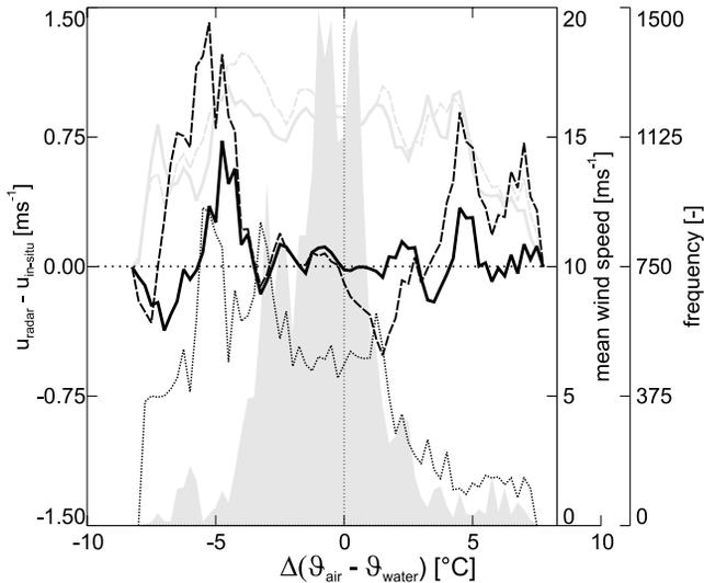
**Figure 13.** Bias (black curve) and standard deviation (shaded curve) of radar retrieved wind speeds (with/without considered air-sea temperature difference (solid/dashed curves)) and in situ wind speeds over air-sea temperature difference. The dotted black curve gives the mean wind speed for each air-sea temperature difference bin. A histogram (shading) of all training/test data sets is plotted.
