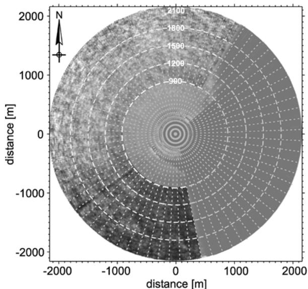
**Figure 4.** Mean RCS of a radar-image sequence of 32 images from Ekofisk 2/4 k. The masked area was not considered for the wind retrieval. The polar image is divided into subareas in range (300 m) and azimuth (5°).
