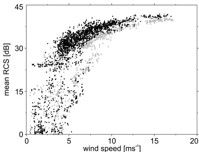
**Figure 3.** Scatterplot of in situ wind speed versus mean RCS. Black dots represent mean RCS from data sets acquired at wind directions between 170° and 40°, while shaded triangles represent data between 40° and 170°.
