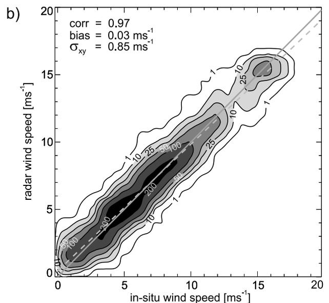
**Figure 11.** Scatterplots giving the comparison of the wind anemometer wind speeds (mean of 10 min) versus wind speeds retrieved from colocated nautical radar images. The radar wind speeds were retrieved in both cases using a NN with the intensity of the mean radar image and the wind direction from the colocated anemometer data as input. In (Figure 11b, additionally, the air-sea temperature difference has been considered for NN training.
