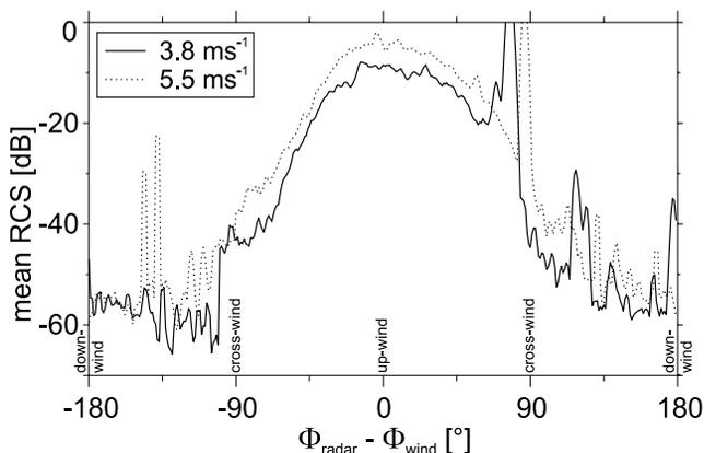
**Figure 2.** Wind direction in respect to radar look direction versus range-integrated RCS for different wind speeds. The data were acquired from a tower-based radar in the Odra Lagoon at the German coast of the Baltic Sea.
