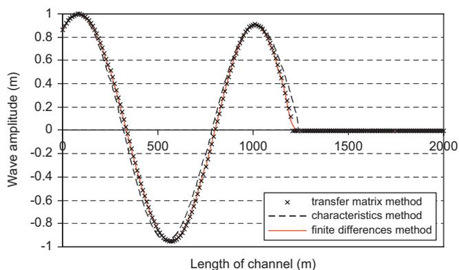
Fig. 5. Comparison of the results obtained by TMM, CM and FDM for  $t = 80$  s.
