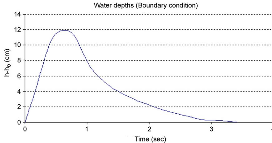
Fig. 6. The variation of water depth value at the first cross-section (boundary condition).
