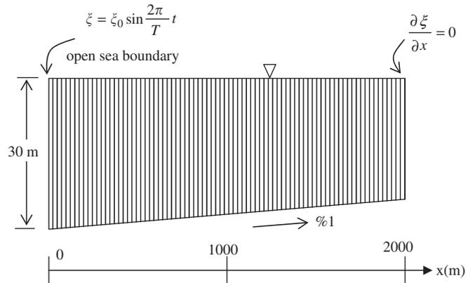
Fig. 1. Wave propagation in the channel.
