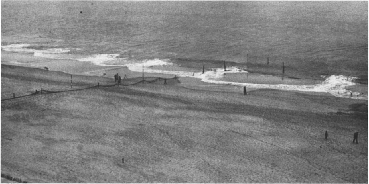
Fig. 5. Photograph of rip currents observed at the Isle of Sylt on November 13, 1976. The Technical University of Braunschweig installed the instrumented profile located at the center of picture.
