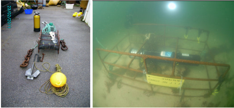
Figure 4.13: Equipment used in the assembly (on the left photo) and sensor on the seabed (on the right photo).
