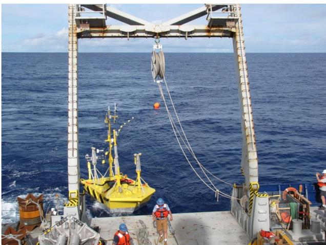
**Fig. 1** EASI buoy off the stern of the R/V Roger Revelle after deployment during the 2010 ITOP experiment
