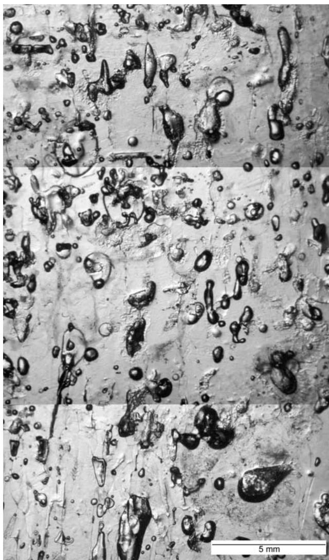
**Figure 7.** Composite micrograph illustrating the inclusion structure of the fine-grained band at the top of the sheet, as viewed in a vertical thin section. Most of the large objects are drained brine inclusions.
