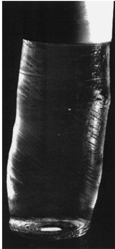
Fig. 6. Photograph of an ice single crystal after straining. This specimen was oriented with the basal planes at 45^\circ to the loading direction (easy glide orientation), and the slip bands are evident on the specimen surface.
