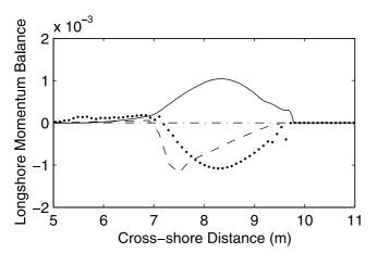
**Figure 4.** Alongshore momentum balance: solid line, the bottom friction; dotted line, the cross-shore gradient of the radiation shear stress  $\left(\frac{\partial S_{yx}}{\partial x}\right)$  given by the Boussinesq model; and dashed line,  $\frac{\partial S_{yx}}{\partial x}$  given by REFDIF.
