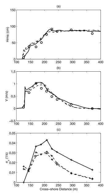
**Figure 19.** Comparisons of the computational results and the field measurements in the cases of regular waves (solid lines), narrow-banded spectrum (dot-dashed lines), and broadbanded spectrum (dashed lines): (a) root mean square wave height, (b) cross-shore distribution of longshore current, and (c) standard deviation of the instantaneous vorticity. Circles, measurements; and crosses, gage locations.
