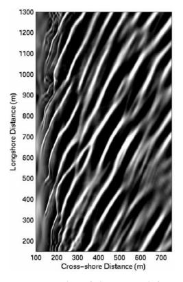
**Figure 14.** A snapshot of the computed free surface elevation at FRF: light areas represent the wave crests of the narrow-banded wave field.
