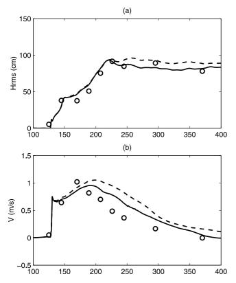
**Figure 10.** Comparisons of the computational results and the field measurements in the case of regular waves: (a) root mean square wave height and (b) cross-shore distribution of longshore current. Solid lines, type 2 of f; dashed lines, type 3 of f; and circles, measurements.
