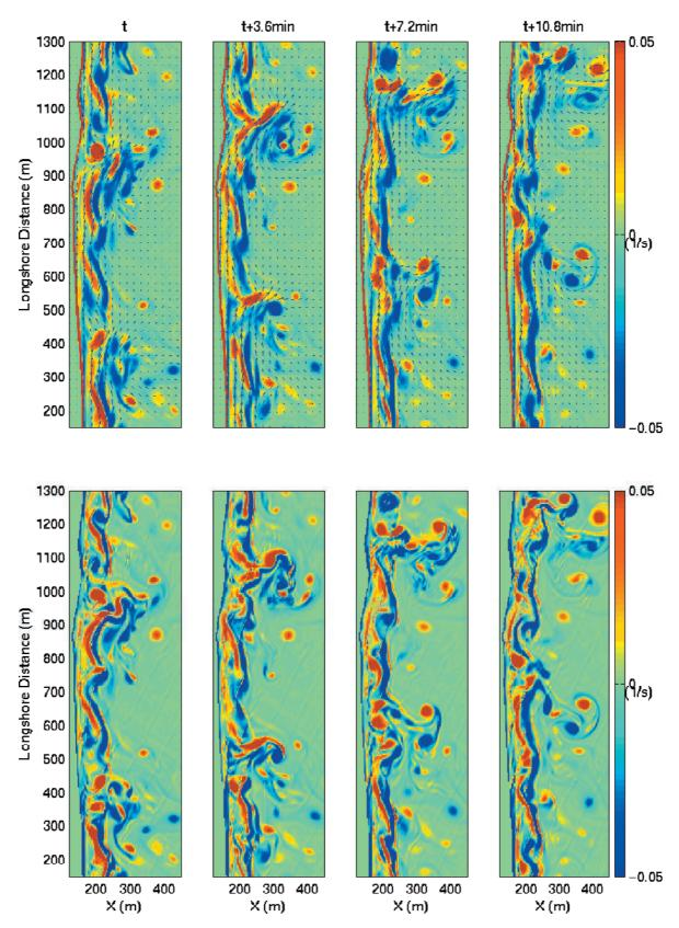
**Figure 11.** Time sequence of the vorticity field. (top) Velocity vectors and vorticity field averaged over 5 peak wave periods and (bottom) instantaneous vorticity field. The faint diagonal streaks are the individual wave crests.
