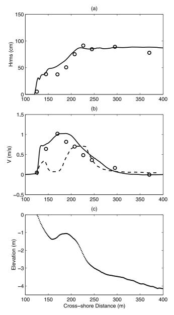
**Figure 15.** Comparisons of the computational results and the field measurements in the case of a narrow-banded spectrum: (a) root mean square wave height, (b) cross-shore distribution of longshore current, where the dashed line depicts the solution of the 1-D model given by *Church and Thornton* [1993], and (c) beach profile.
