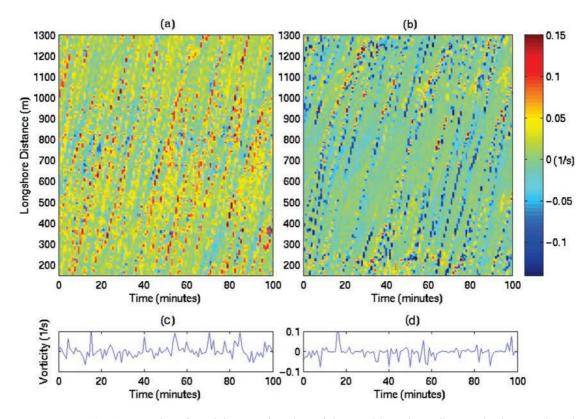
**Figure 12.** (a) Contour plot of vorticity as a function of time and longshore distance in the trough and (b) seaward of the bar crest and (c) time series of vorticity at the measurement array in the trough and (d) seaward of the crest.
