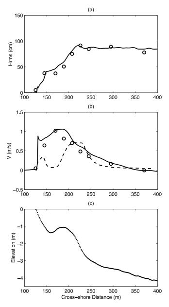
**Figure 9.** Comparisons of the computational results and the field measurements in the case of regular waves and type 1 bottom friction: (a) root mean square wave height, (b) cross-shore distribution of longshore current, where the dashed line depicts the solution of the 1-D model given by *Church and Thornton* [1993], and (c) beach profile.
