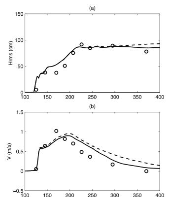
**Figure 16.** Comparisons of the computational results and the field measurements in the case of a narrow-banded spectrum: (a) root mean square wave height and (b) cross-shore distribution of longshore current. Solid lines, type 2 of f; dashed lines, type 3 of f; and circles, measurements.
