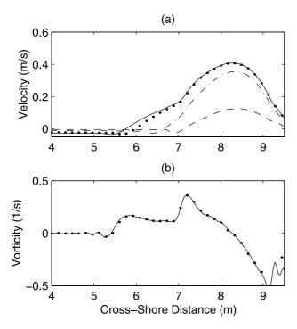
**Figure 2.** Cross-shore profiles of (a) the computed longshore currents at t = 20 s (dashed line), 50 s (dashed line), 100 s (dotted line), and 120 s (solid line) and (b) the vorticity obtained from the mean current (solid line) and the instantaneous fluid particle velocity (dotted line).
