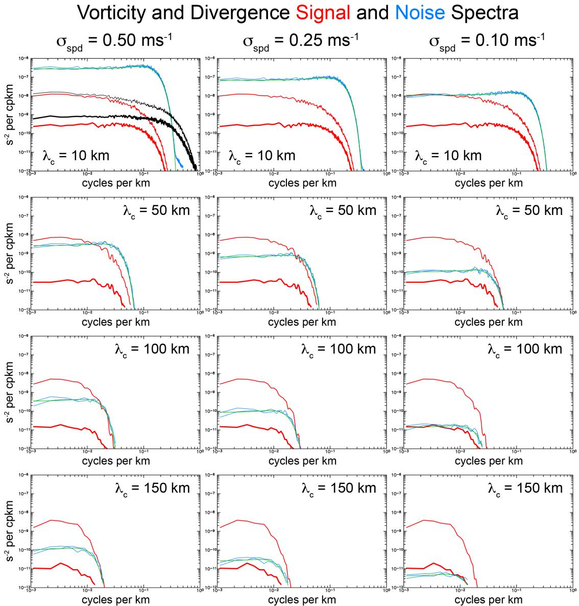
370 FIG. 4. Along-track wavenumber spectra of the noise of divergence and vorticity computed from velocity
