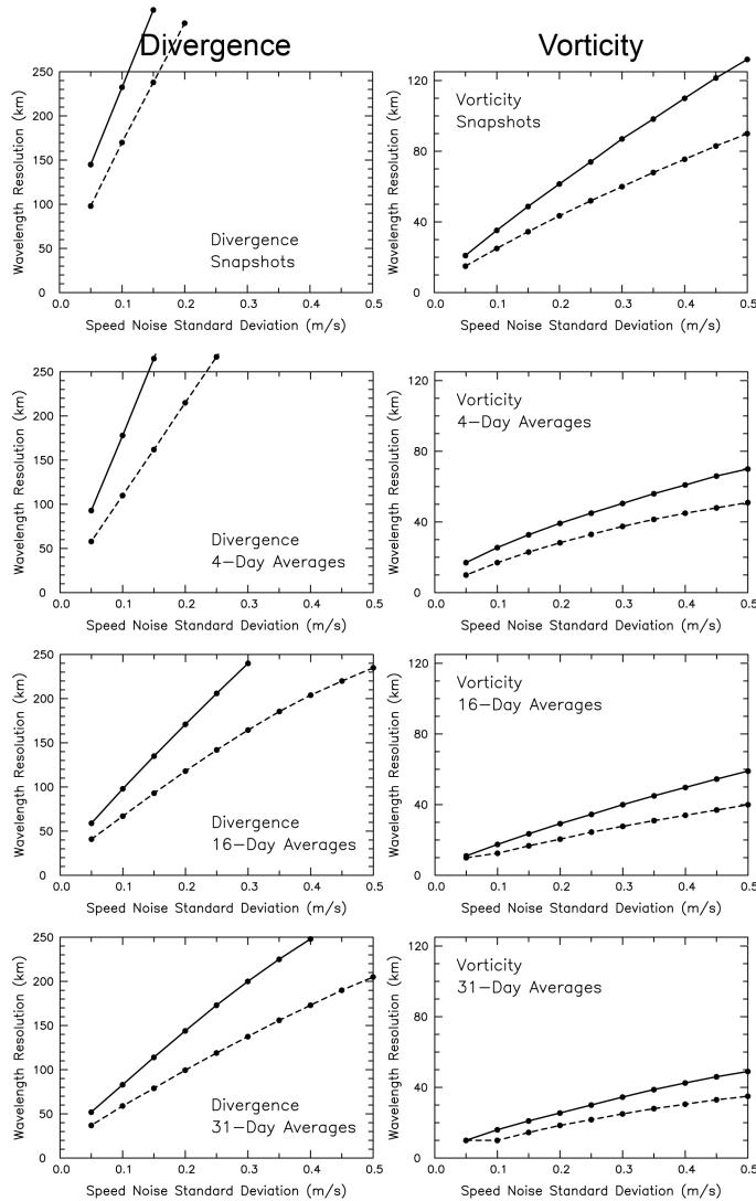
526 FIG. 8. The resolution capabilities of WaCM estimates of divergence (left column) and vorticity (right column)
