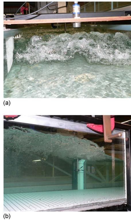
FIG. 9. (Color online) Photographs of breaking bore roller (shutter speed: 1/80 s). Laboratory data:  $d = 0.14$  m,  $Fr = 1.5$ . (a) Looking at incoming bore roller. (b) Underside of the bore roller showing the entrained air bubble-bore propagation from left to right.
