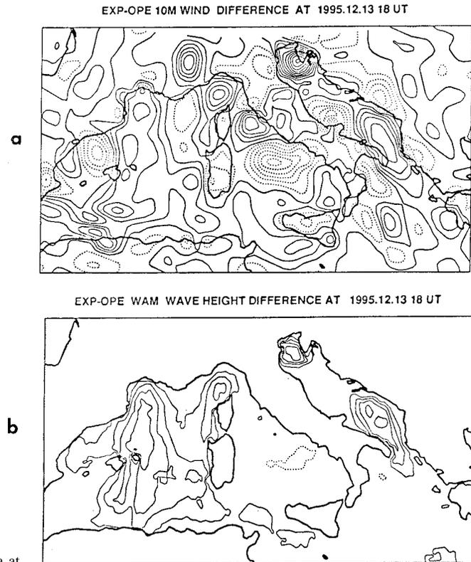
FIG. 14. With reference to Fig. 13a wind speed differences obtained with reduced and normal horizontal diffusion. Isolines at  $20 \text{ cm s}^{-1}$  interval. Continuous lines represent positive values; dotted lines are for negative ones. (b) As in (a) but for wave height. Isolines at 5-cm interval. (After Cavaleri et al. 1997.)
