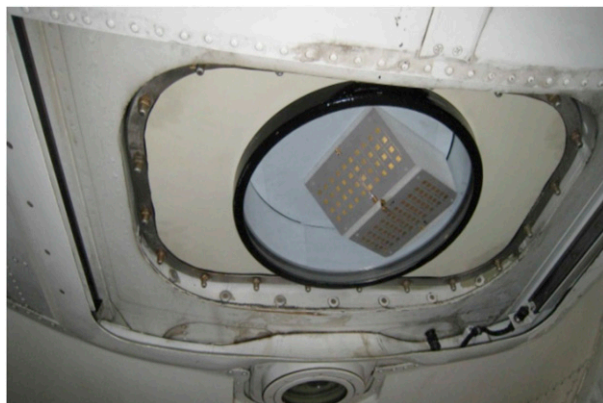
FIG. 6. External view of both antennas aiming through the quartz windows.
