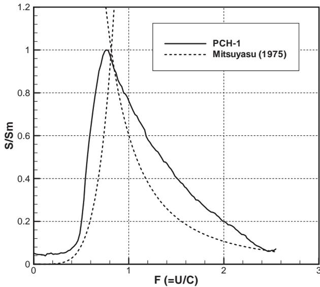
Fig. 6. Overlap of the curve of the spreading function obtained in PCH-1 and the Mitsuyasu [8] one.
