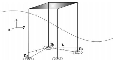
Fig. 2. Scheme of the directional wave meter.
