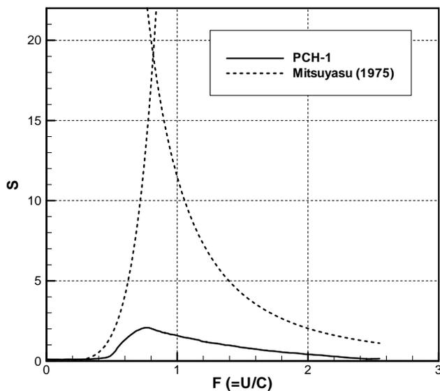
Fig. 7. Curves of the absolute spreading function from PCH-1 and of the estimated formulation of Mitsuyasu [8] for an average wind speed of 8.0 m/s.
