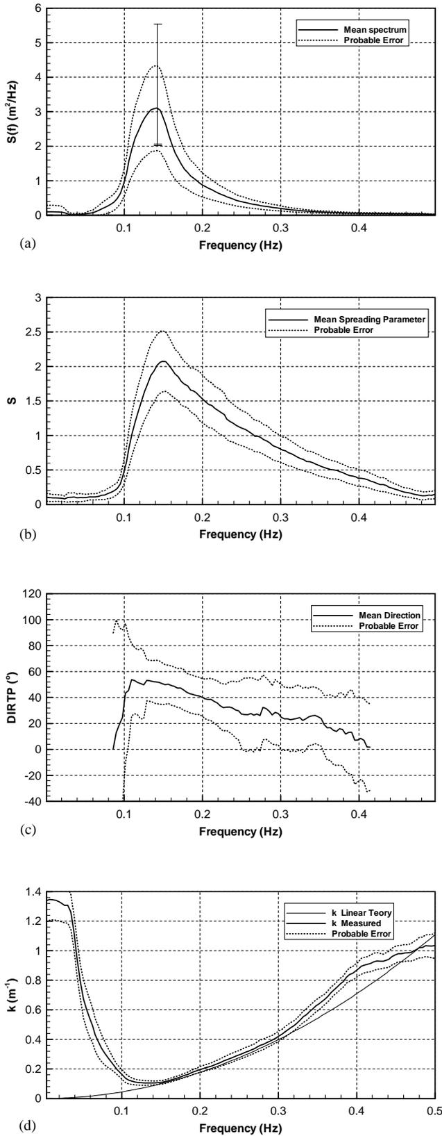
Fig. 3. (a) Power spectrum. The error bar shows the 90% confidence limit at the peak frequency. (b) Angular spreading parameter. (c) Direction. (d) Wave number.
