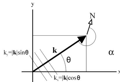
Fig. 1. Representation of the wave number vector and its projections onto the coordinate system.  $\alpha$  is the direction of the wave referred to true North.
