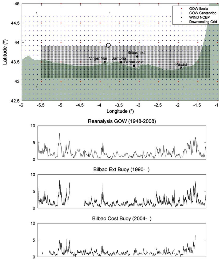
Fig. 2. Reanalysis databases and instrumental data available in the area of interest and the downscaling grid proposed to obtain coastal waves.
