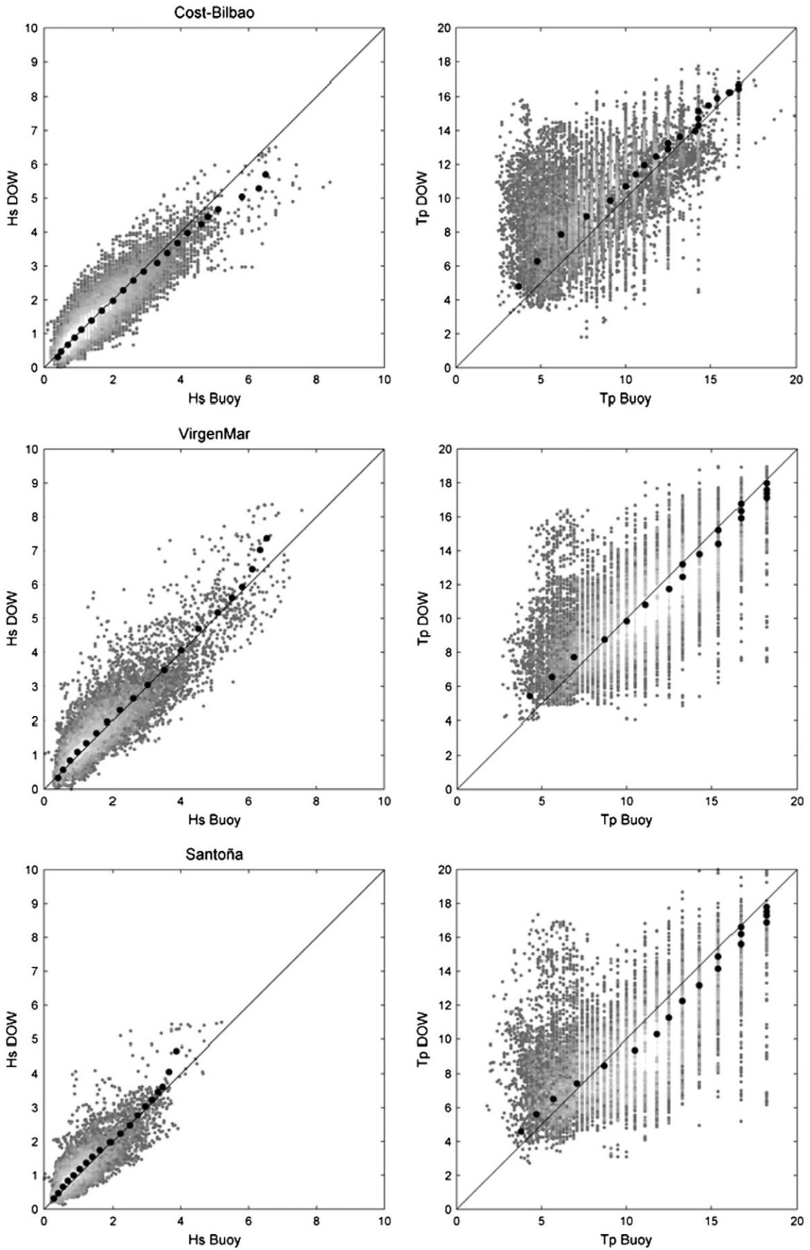
Fig. 12. Scatter diagrams of measured versus modeled  $H_s$ ,  $T_p$  at Cost-Bilbao, Virgen del Mar, Santoña buoys.
