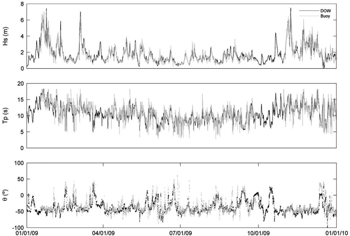
Fig. 11. Comparison between reconstructed and measured  $H_s$ ,  $T_p$  and  $\theta_m$  at Virgin Mar buoy 2009.
