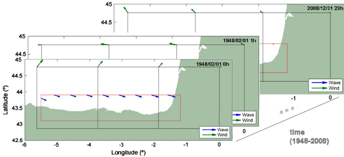
Fig. 6. Time series of the computational conditions (wave data along the grid boundaries of the wave computational model and wind data from the NCEP/NCAR database).
