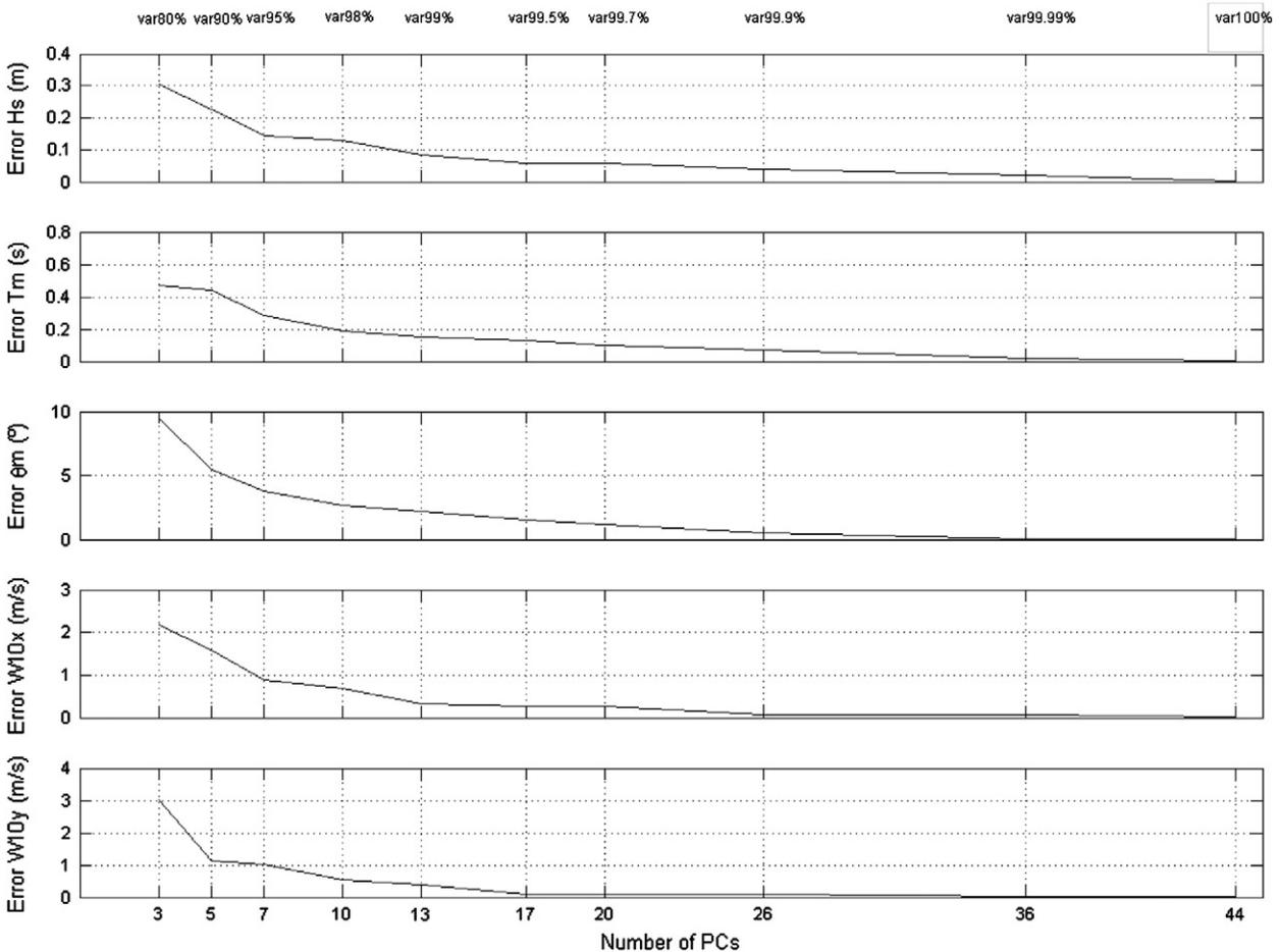
Fig. 7. Root mean square error of the variables that define the grid boundaries as a function of the explained variance.
