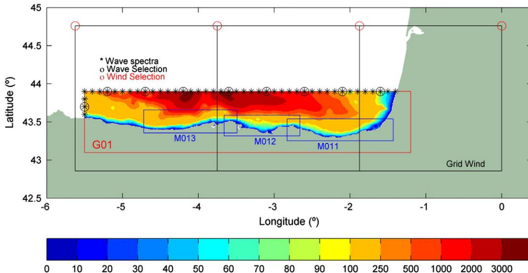
Fig. 5. Downscaling grids: G01 (0.01°×0.008°) and M011, M012, M013 (0.005°×0.004°). NCEP/NCAR wind grid (~1.875°) associated to wave propagations. The directional spectra at the boundaries of the computational (each 0.1°), the wave data and wind data considered in the definition of the computational conditions in the selection process. Bathymetry of the downscaled area (depth in m).
