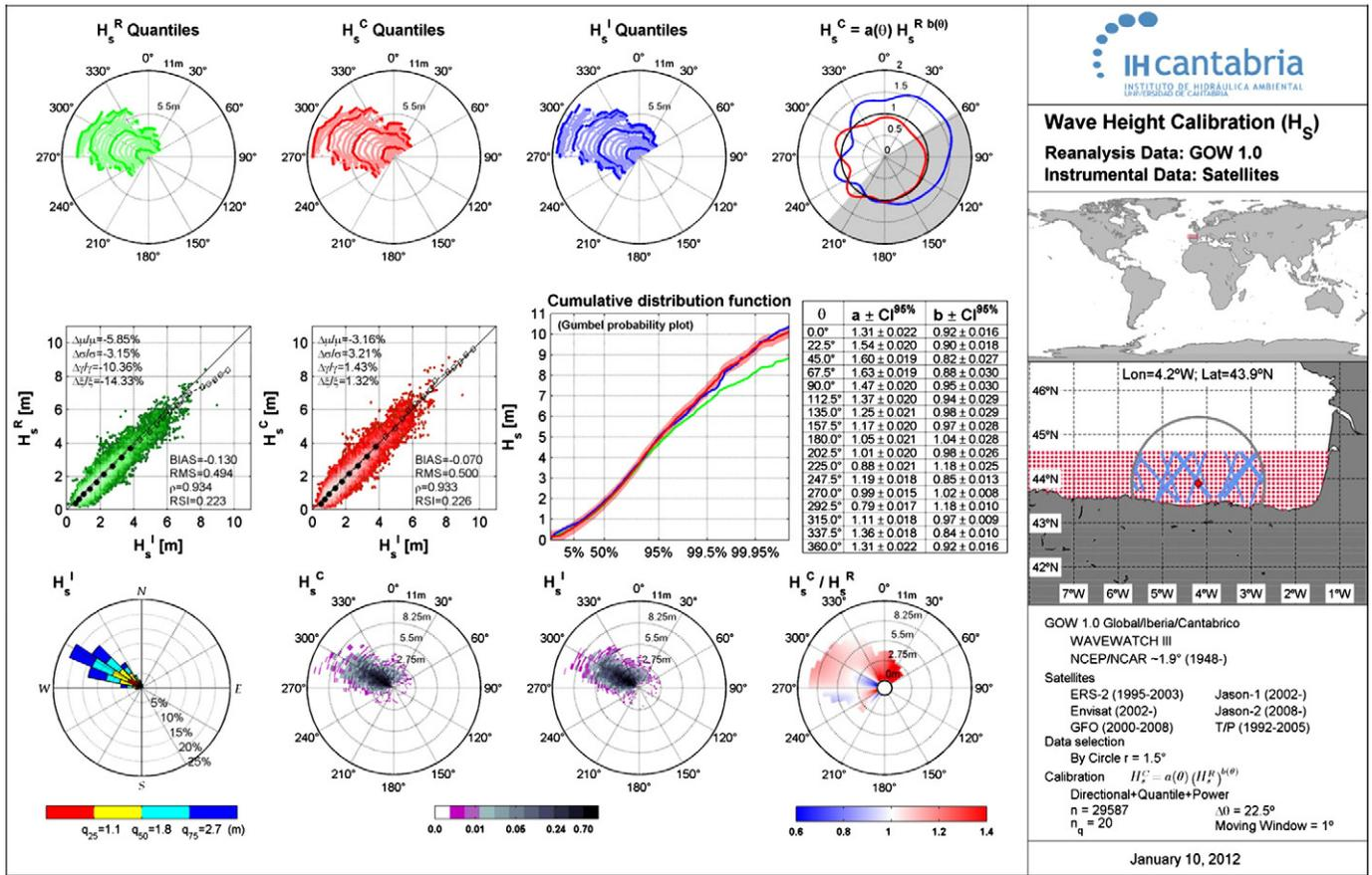
Fig. 3. Significant wave height GOW calibration with satellite data (Mínguez et al., 2011a). Instrumental data in blue, reanalysis data in green and calibrated data in red.
