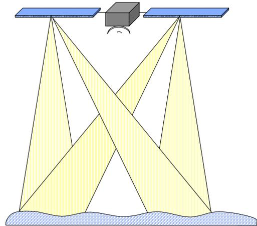
Figure 1. Wide Swath Ocean Altimeter - Standard Configuration
