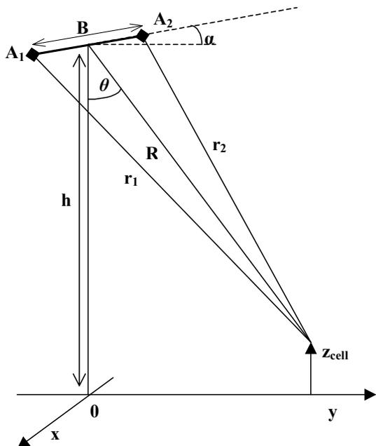
Figure 3. Geometry of Across-Track Interferometry
