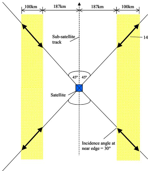
Figure 2. Full “Wavemill” swath configuration
